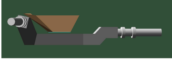
Fig. 5 Three-dimensional illustration of under-crossing concrete encased structure.
