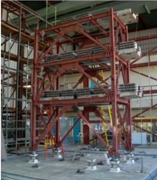
Figure 4 Test of 3-Story Isolated Building
