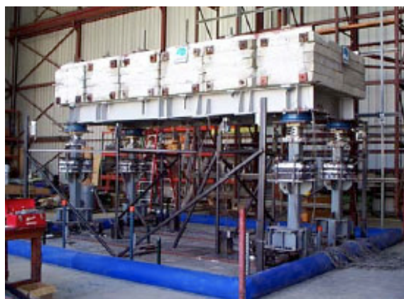
Figure 6 Shaking table test specimen of simple supported bridge with different substructure stiffness
