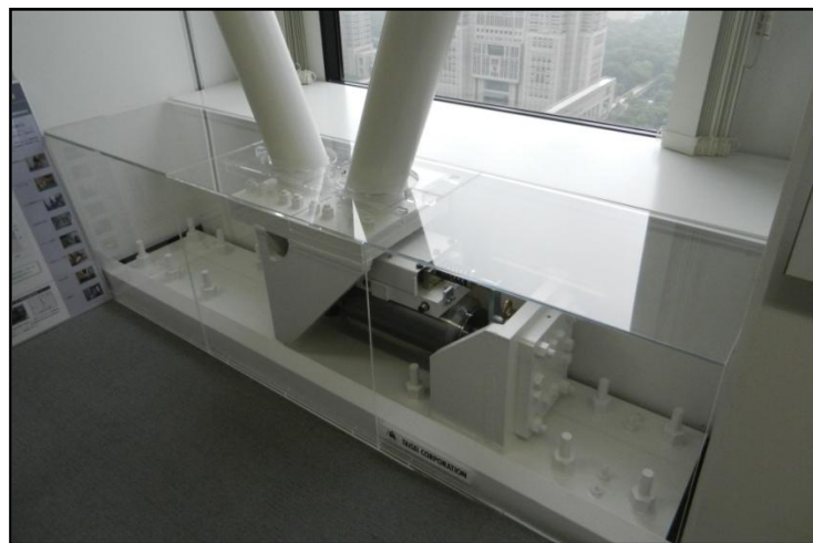
Fig. 4 Retrofit damper at 54-story Shinjuku Center Building
