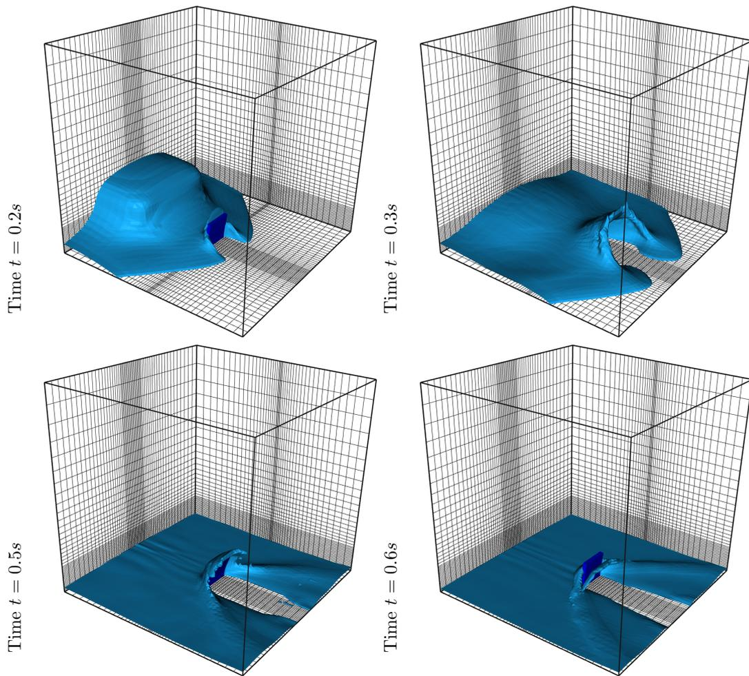
Figure 3: Tri-dimensional dam break problem. Evolution of the free surface and motion of the structure.
