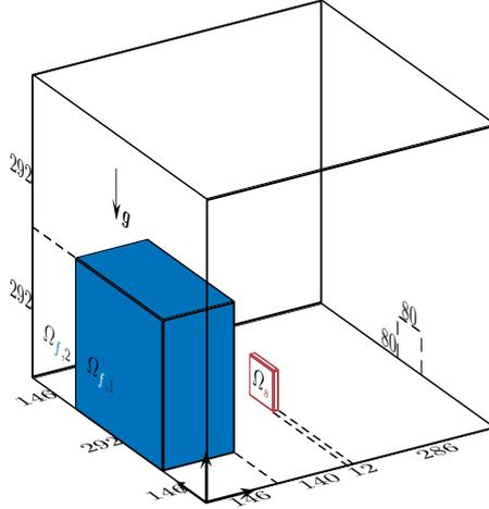
Figure 1: Three-dimensional water column impacting an obstacle: geometry (given in  $mm$ ) and boundary conditions
