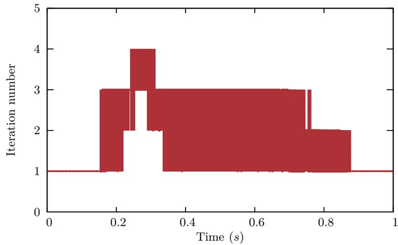
(a) Number of iterations in order to make the DFMT-BGS algorithm converge for the three-dimensional dam-breaking problem
