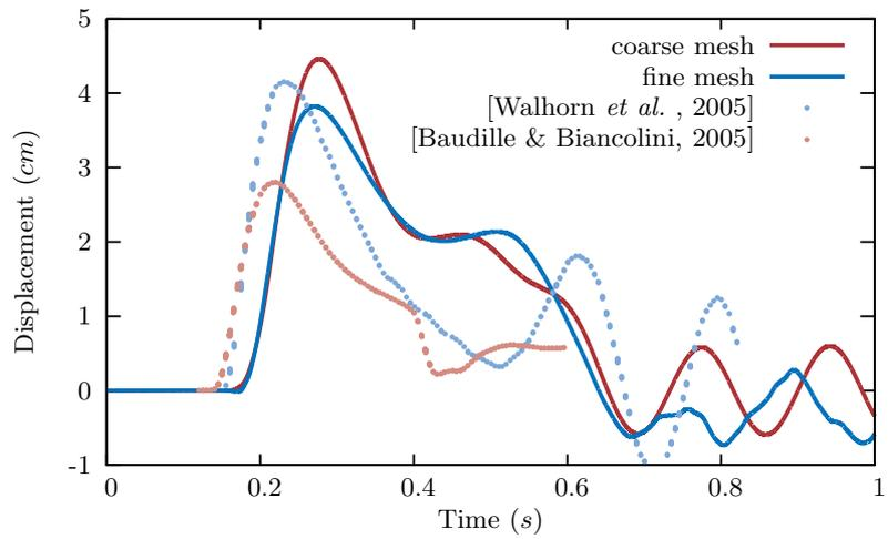
(b) Three-dimensional dam break example: obstacle displacement in  $e_x$  direction of center point of the top face (40; 6; 80) and comparison with 2D models [Baudille & Biancolini, 2005, Walhorn et al., 2005]
