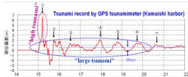
Fig.2 Superposition of "large tsunami" and "high tsunami" in the Tohoku-Pacific Earthquake (PARI)
