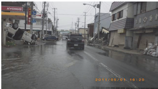
Fig. 4 Inundation and low ground level caused by coseismic subsidence (in Miyagi Prefecture)
