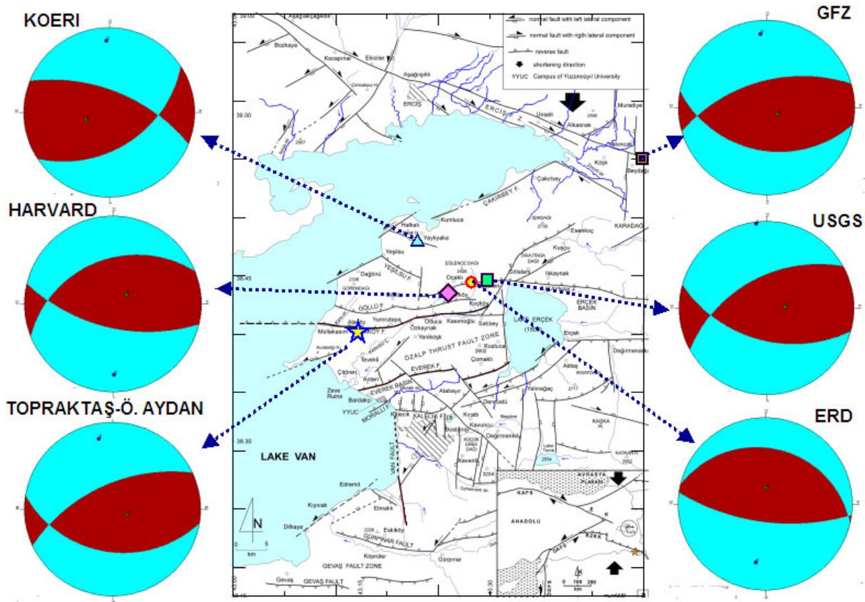
Fig. 3 Faults mapped by Koçyiğit et al. (2011) and focal mechanism solutions by various institutes
