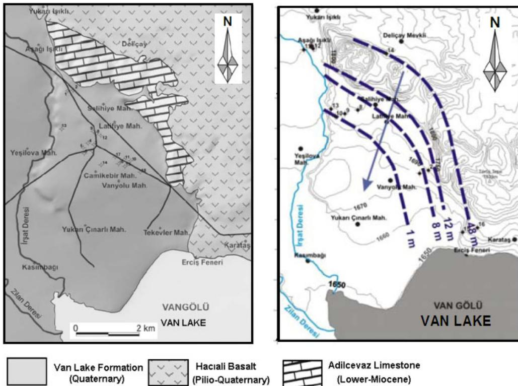
Fig. 2. Geology and hydrogeology of Erciş Plain (re-arranged from Özvan et al., 2008)
