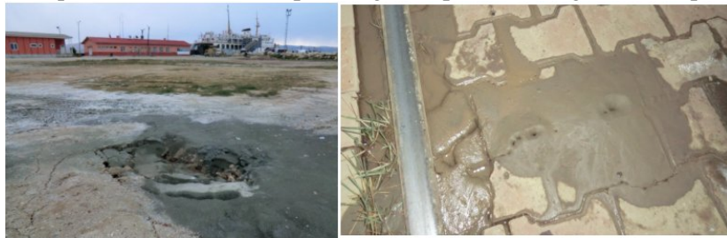
(b) Liquefaction and lateral spreading at Topraktaş village (Karasu plain)
