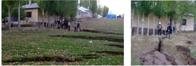
(a) Liquefaction and lateral spreading at Çelebibağı (Erciş)
