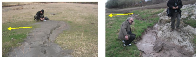
(b) Liquefaction and lateral spreading at Topraktaş village (Karasu plain)
