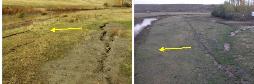
(a) Liquefaction and lateral spreading at Çelebibağı (Erciş)
