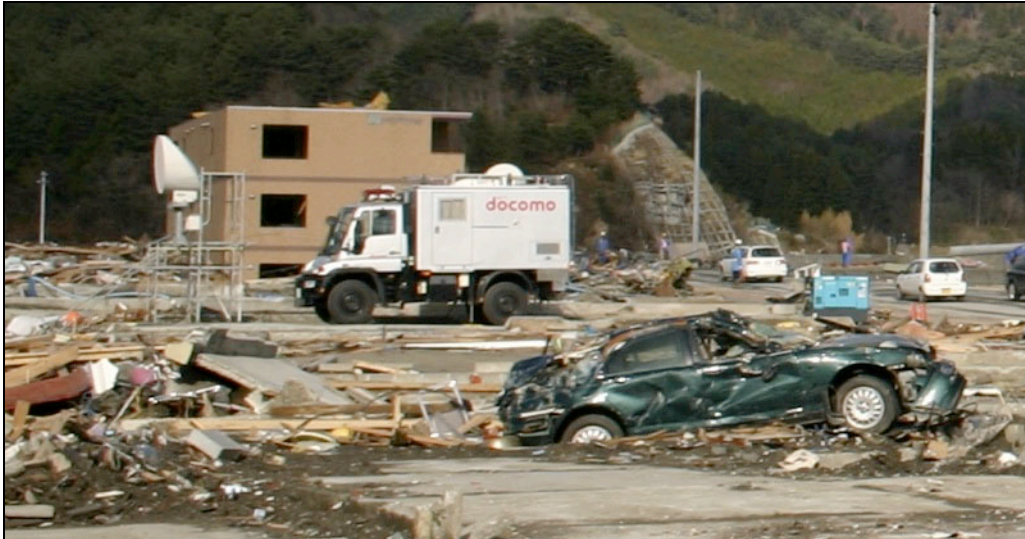
Figure 21. A temporary microwave repeater in the town of Otsuchi
