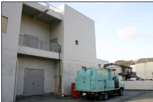
Figure 5. Left: A portable genset at Kamaishi CO with a truck of additional diesel storage expecting very long autonomies. Right: Watertight door at Kamaishi CO.
