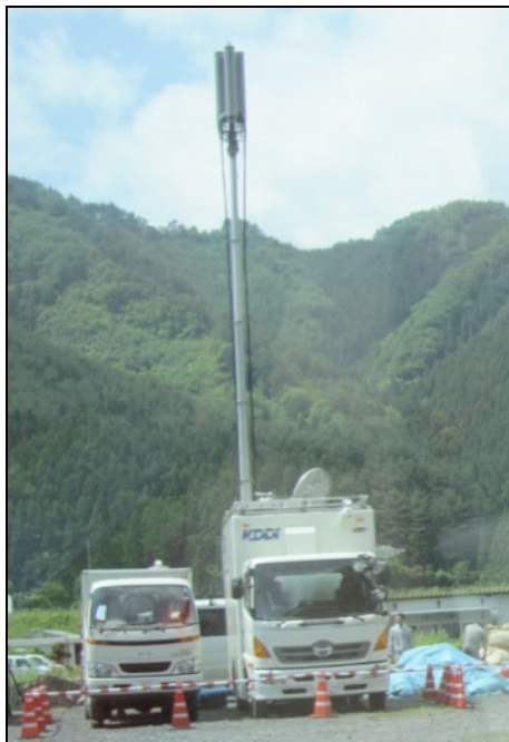
Figure 18. COW in place to restore coverage
