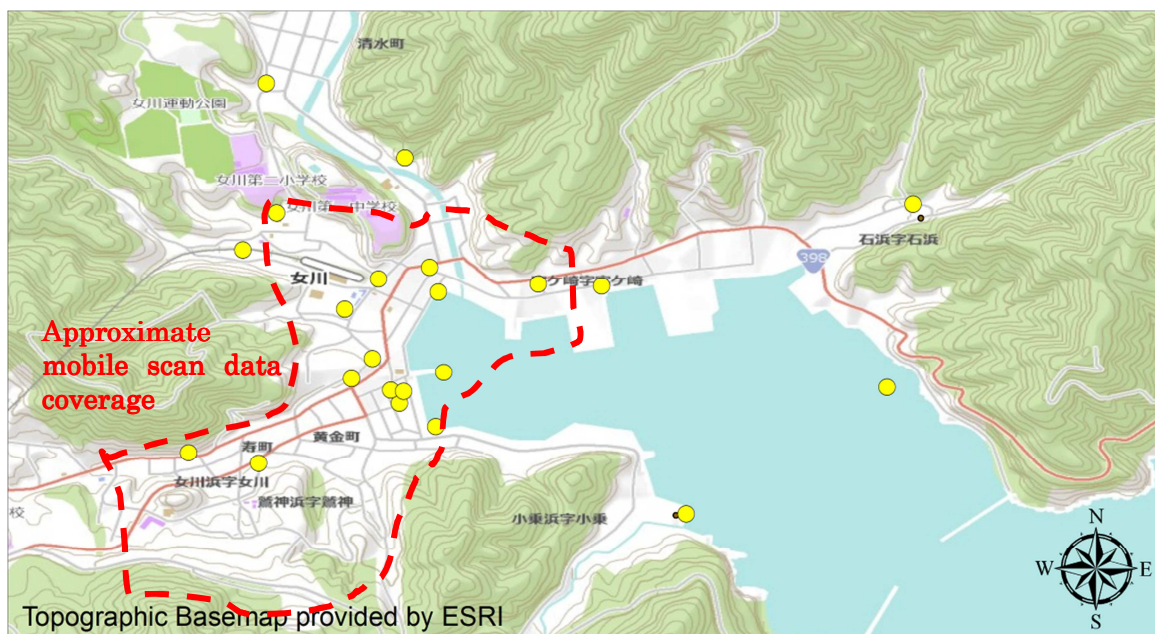
Fig. 5 Scan locations (yellow circles) in Onagawa for topographic mapping. The red-dashed line represents the approximate extents of mobile laser scan data provided by Asia Air Survey, Co.
