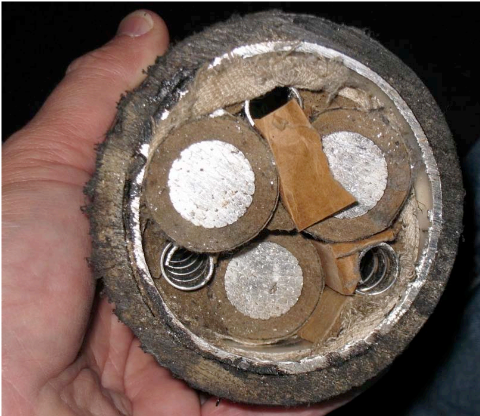
Figure 6. Oil-Type Cable Cross Section
