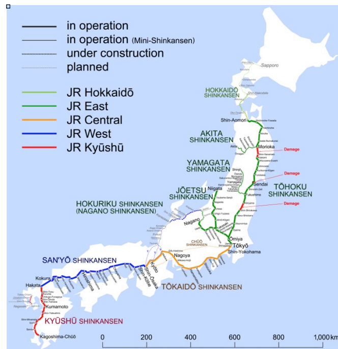
Fig. 16 Map of Shinkansen with locations of damage during earthquake
