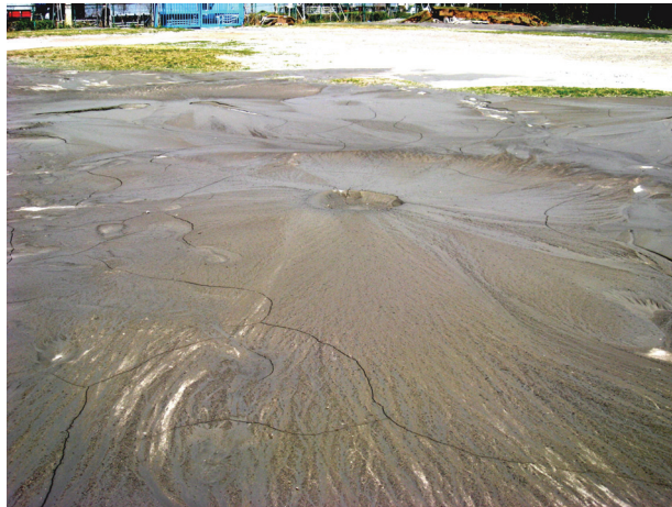
Photo 1 Sand boils observed in Shin-Kiba area
