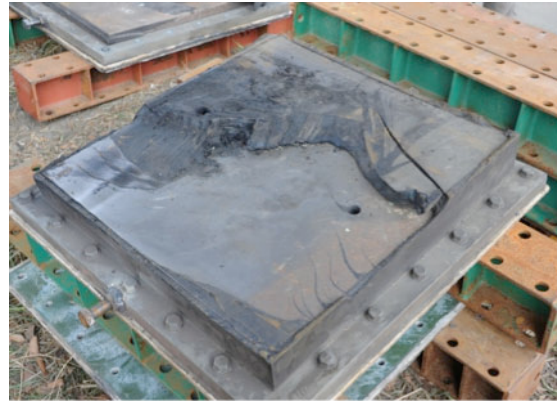
Photo 2 Rupture of elastomeric bearings of Tobu Viaduct
