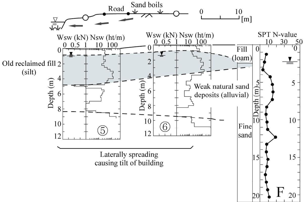
Fig. 12 Results of Swedish weight sounding tests at Jukken-gawa River (cross section a-a') (The ratios of distance to depth/height are not to scale.)
