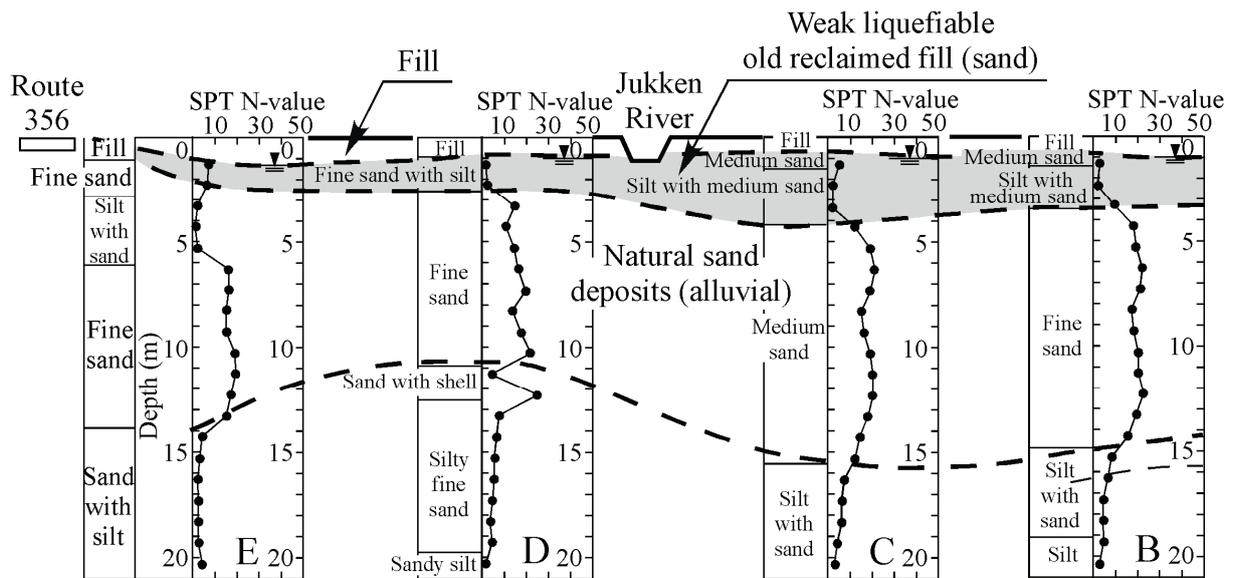
Fig. 14 Soil profile along cross section b'-b'' (The ratios of distance to depth/height are not to scale.)
