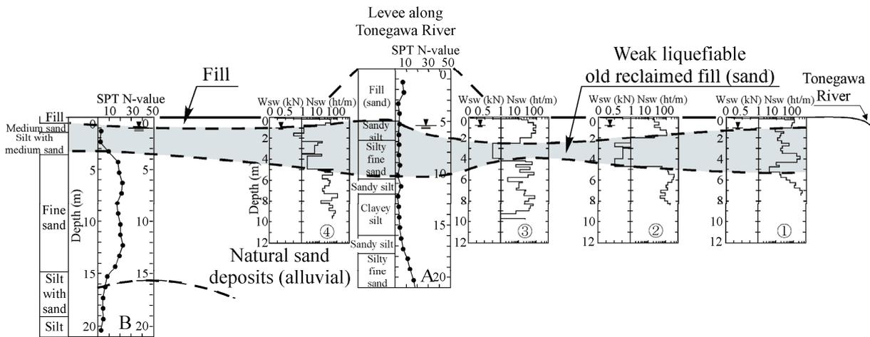
Fig. 13 Soil profile along cross section b-b' (The ratios of distance to depth/height are not to scale.)
