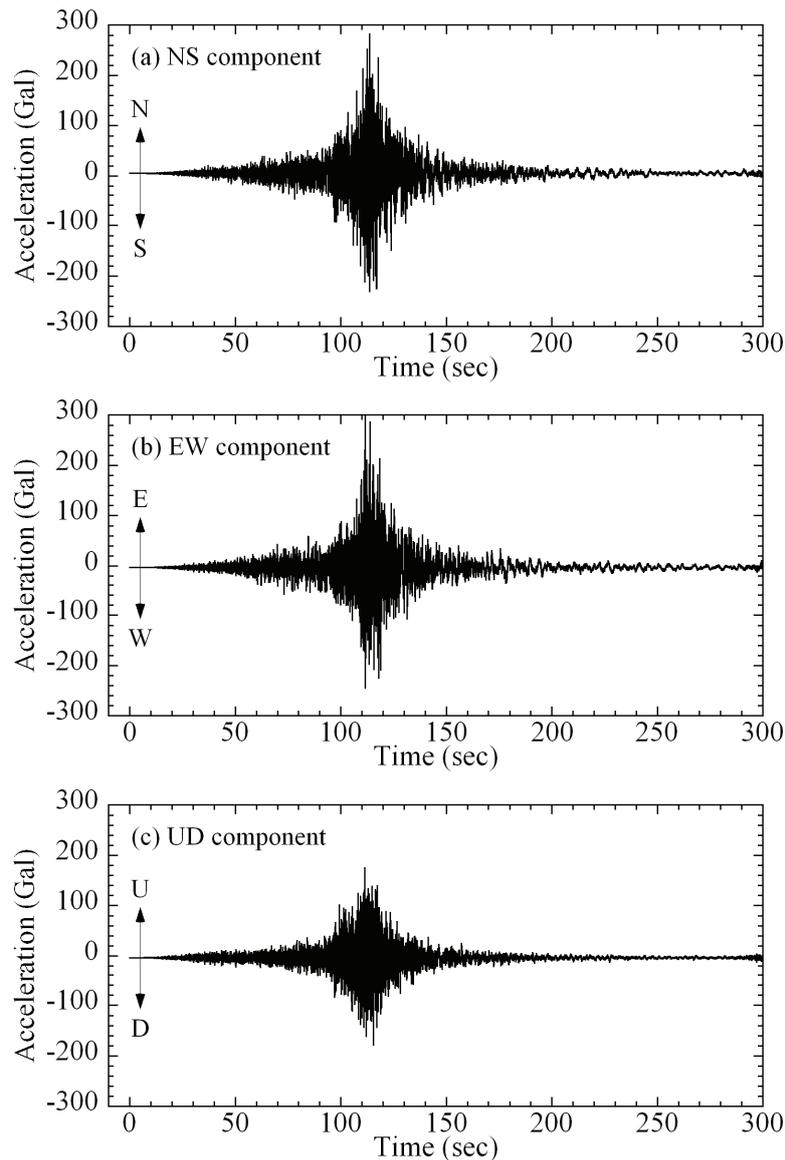
Fig. 3 Acceleration records of the main shock observed at Sawara station of K-Net
