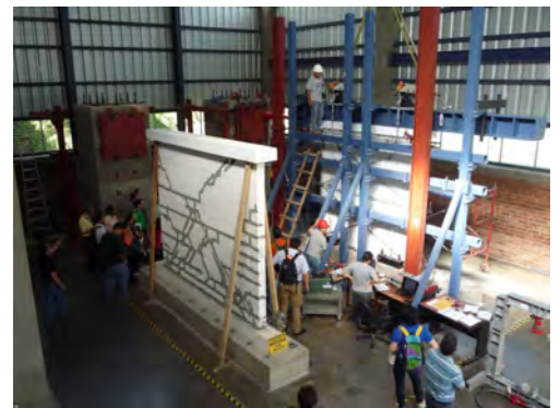
Photo 2 Preparation of loading at structural laboratory in UCA: specimen of real-size confined concrete block masonry.
