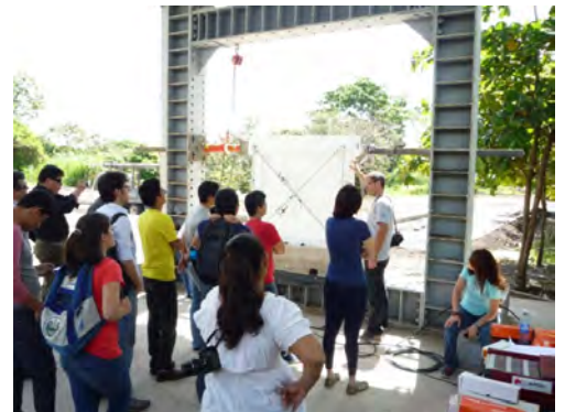
Photo 3 Preparation of loading at structural laboratory in UES: a wall specimen of real-size confined concrete block masonry.
