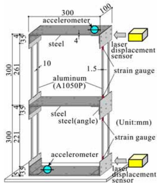
Fig. 1 Experimental specimen for structural collapse.
