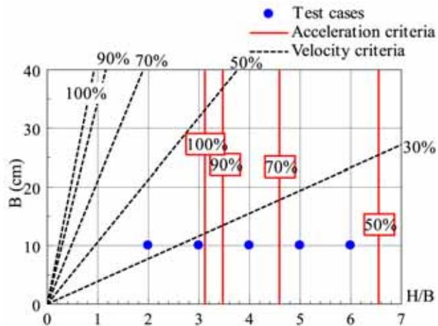
Fig. 9 Relationship between aspect ratio of rectangular specimens and overturning criteria [Eq.(3) and (4)]
