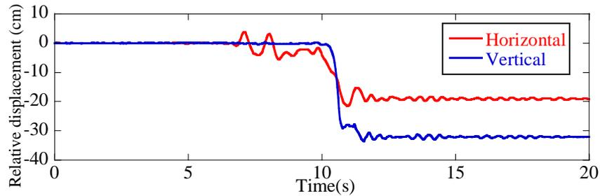
Fig. 7 Relative displacement of top story measured by optical motion tracking (Test #8).
