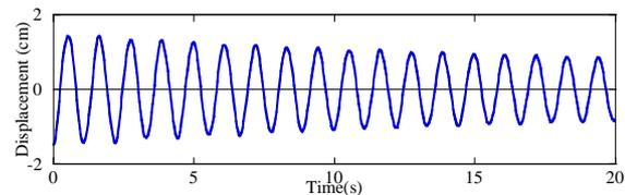
Fig. 2 Displacement of top floor in a free vibration test.
