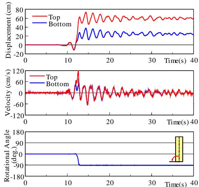
Fig. 10 Time histories of horizontal displacement, horizontal velocity and rotational angle of a rectangular specimen measured by vision-based motion tracking ( $H/B=5.0$ .100% Taft input)
