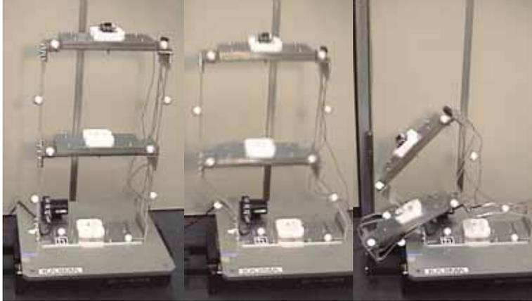
Photo 1 Process of structural collapse during shaking.
