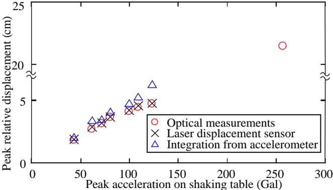
Fig. 4 Comparison of maximum relative horizontal displacement measurements among sensors.
