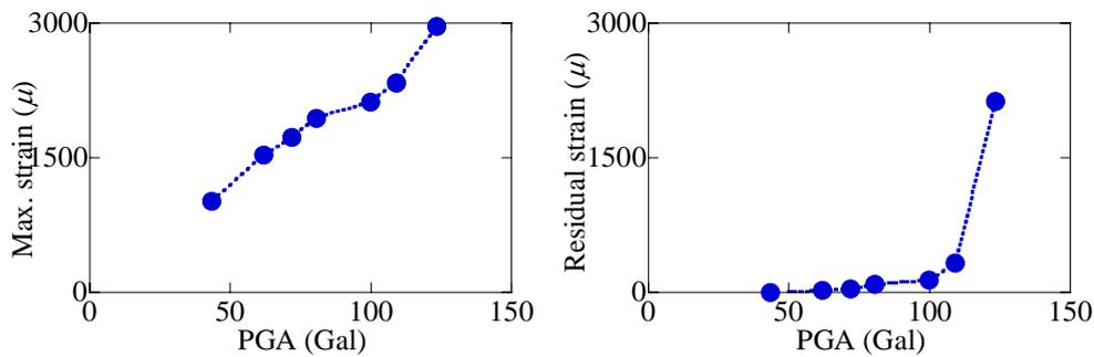
Fig. 5 Strain from gauges at foot of first-story column. Test #8 has no data because strain exceeds the limit of measurements.
