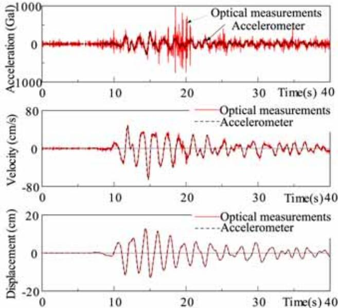
Fig. 8 Comparison of motions on shaking table measured by vision-based motion tracking with accelerometer.
