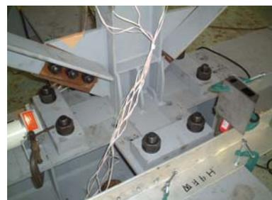
(b) Base plate with four wings of three-story test frame
