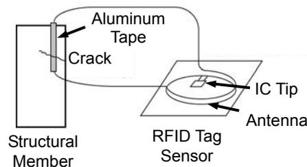
(b) Schematic view of application of RFID tag sensor to the structural members
