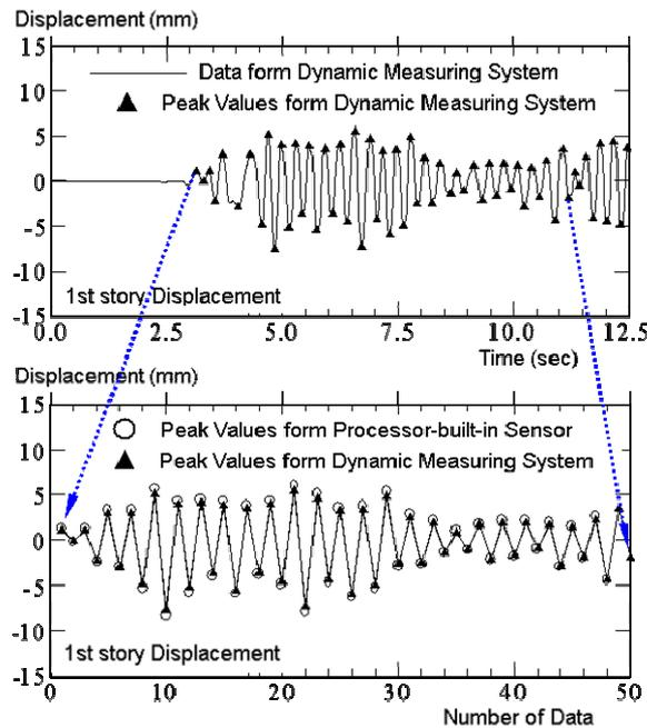
Fig. 15 Comparison of peak data obtained from dynamic measuring system and wiring-saving sensor system
