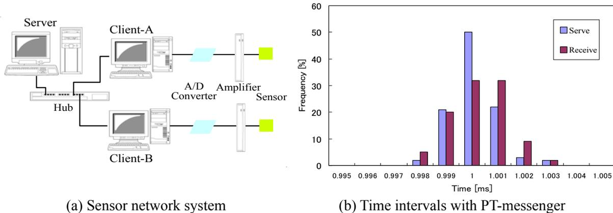
Fig. 17 Experiments of sensor network
