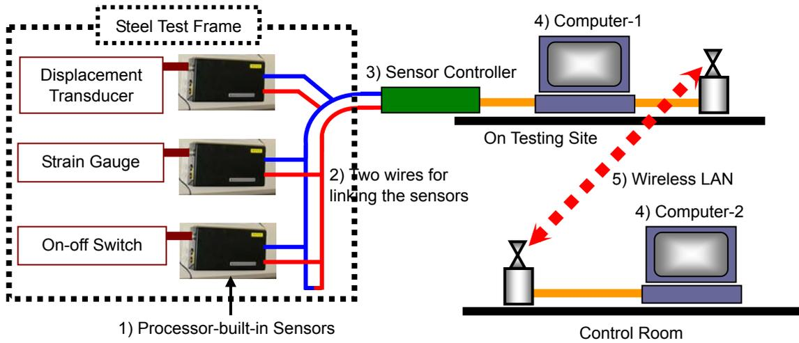
Fig. 13 Composition of wire-saving sensor system for three-story steel frame test
