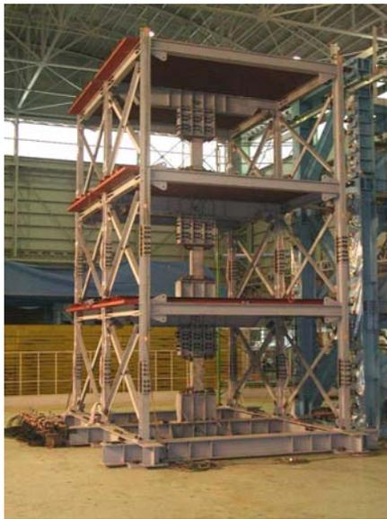
(a) Example of HPFRCC dampers for structural control
