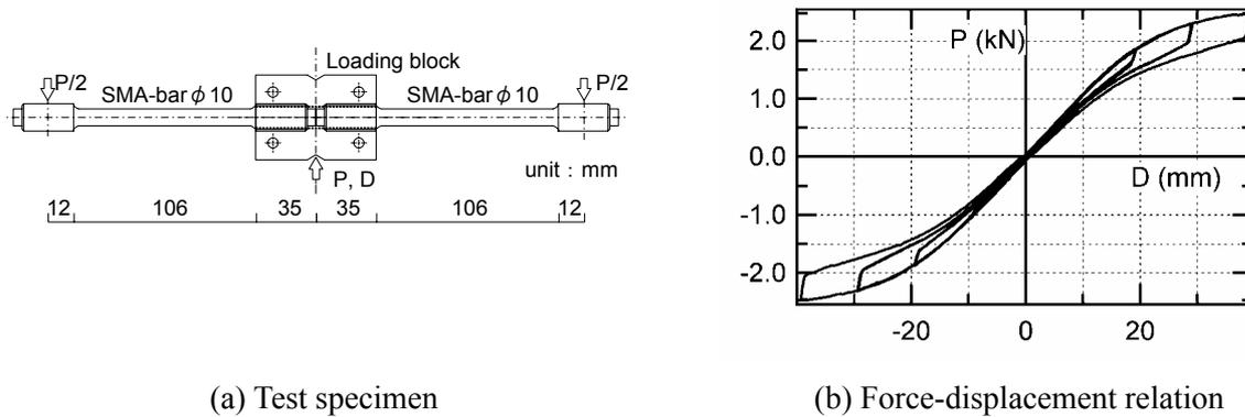
Fig. 21 Bending test on SMA bar
