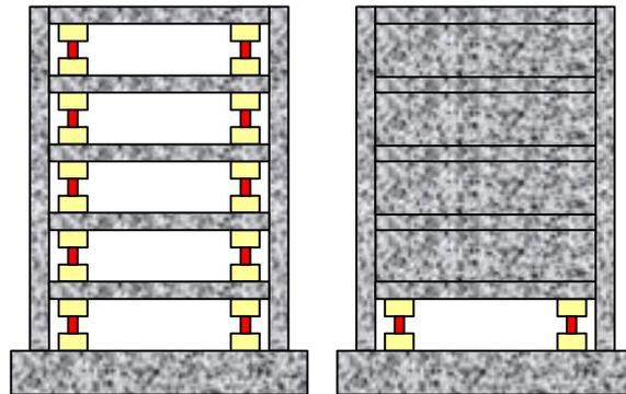
(b) Application examples of HPFRCC dampers in RC structures
