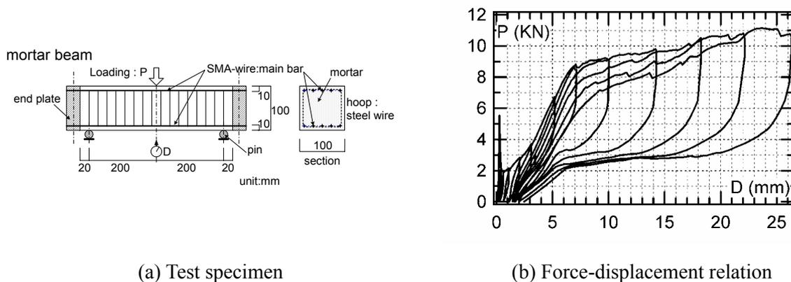
Fig. 22 Bending test on cement mortar beam
