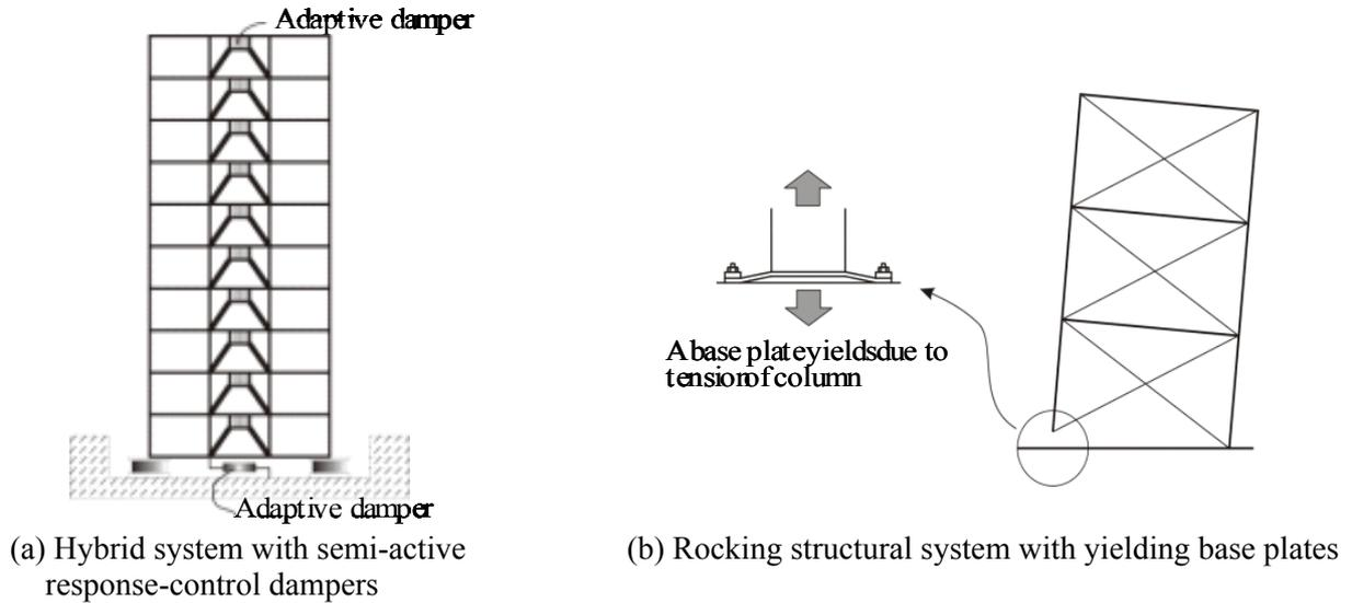
Fig.2 Examples of auto-adaptive structural systems
