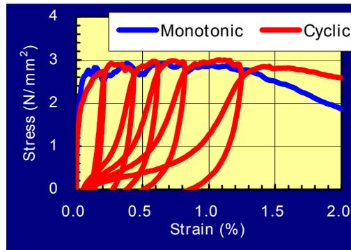
Fig. 29 Material properties of developed HPFRCC
