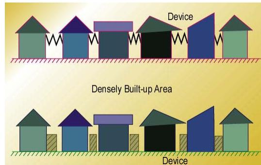
Fig. 6 Retrofit system using loose linking elements
