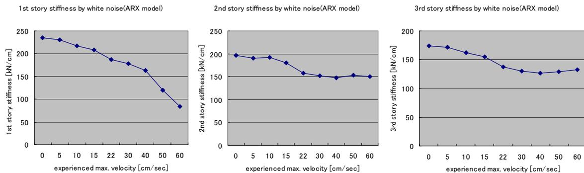
Fig. 11 Stiffness change according to experienced maximum velocity
