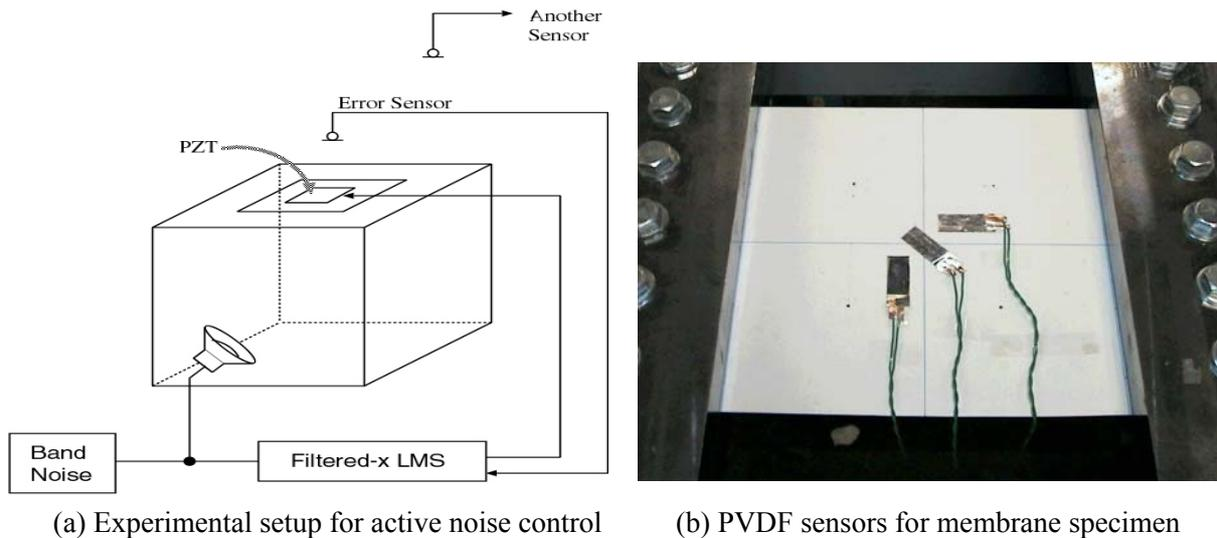
Fig. 27 Application of PZTs and PVDF
