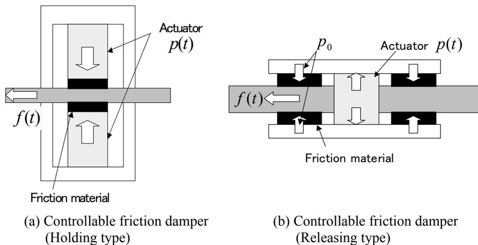
Fig. 26 Two types of friction dampers
