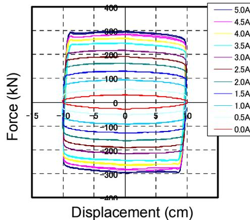
Fig. 25 Force-displacement relationships of 400 kN MR damper
