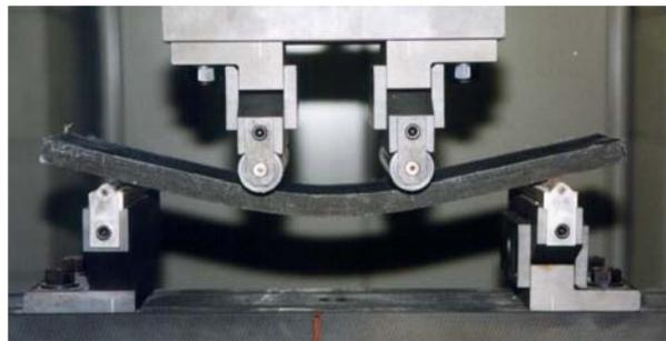
Fig. 28 Flexural test of unreinforced HPFRCC plate
