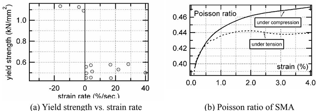
Fig. 20 Characteristics of SMA
