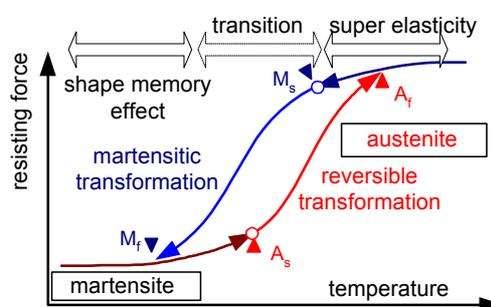
Fig. 18 Material phase-property-temperature relation of SMA
