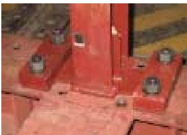
(a) Base plate with two wings of five-story test frame
