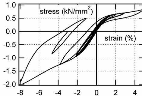
Fig. 19 Stress-strain relation of SMA bar
