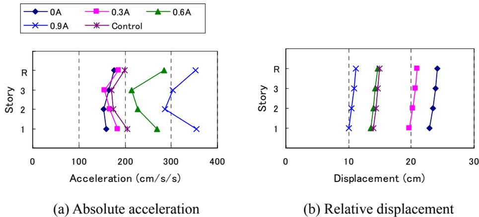
Fig. 24 Average values of response of each story of positive and negative sides (1940 El Centro NS, Maximum velocity is 50cm/s)
