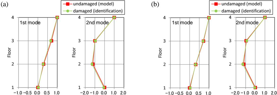
Figure 4.8. Translational mode shapes for undamaged (frame model) and damaged (identification): (a) *TR* direction; (b) *LG* direction
