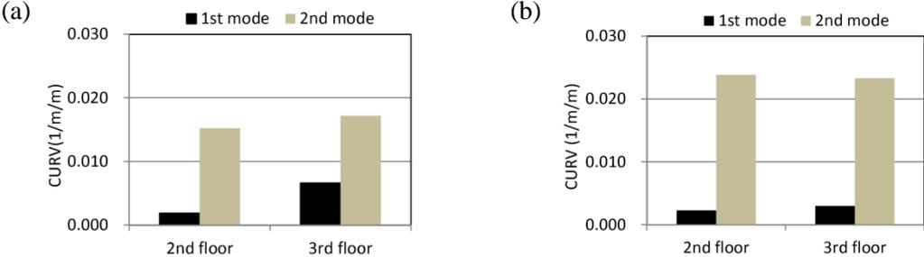
Figure 4.9. Changes in curvature between undamaged mode and damaged mode: (a) *TR* direction; (b) *LG* direction
