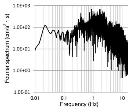
Figure 3.4. Acceleration Fourier spectrum in TR direction at the first floor of NIB
