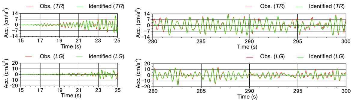
Figure 3.8. Comparison between observed acceleration record and acceleration wave calculated by system identification (on the roof of the NIB)
