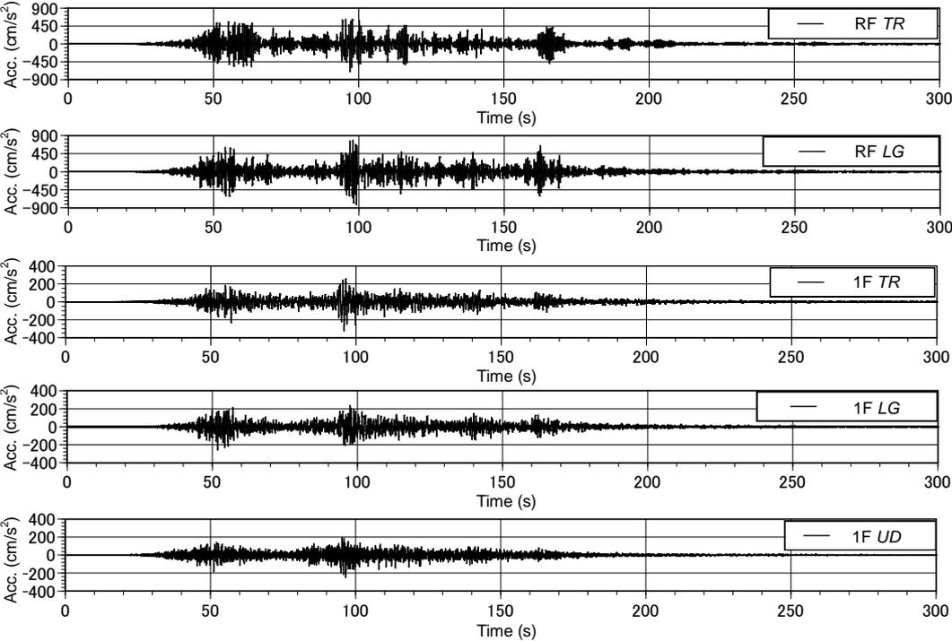
Figure 3.2. Acceleration time history for main shock of the 2011 Tohoku Earthquake observed in the NIB
