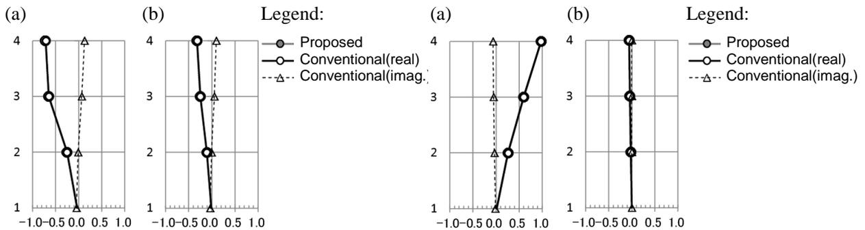
Figure 4.6. Eigenmode at location NE (3.44 Hz): (a) *TR* direction and (b) *LG* direction.
