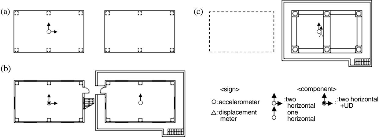
Figure 3.1. Location of observation points used in this study (left: NIB; right: IB): (a) roof, (b) first floor, and (c) basement floor
