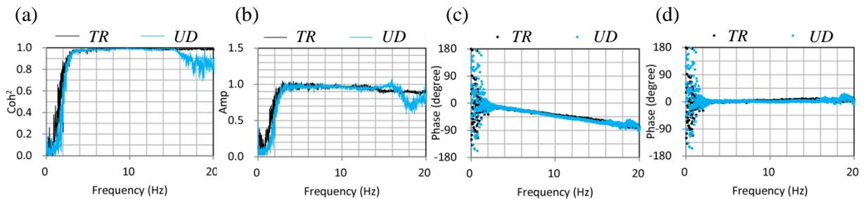
Figure 4.2. Comparison of frequency characteristics between two types of accelerometers: (a) COF, (b) amplitude of FRF, (c) phase of FRF (before time correction), and (d) phase of FRF (after time correction)
