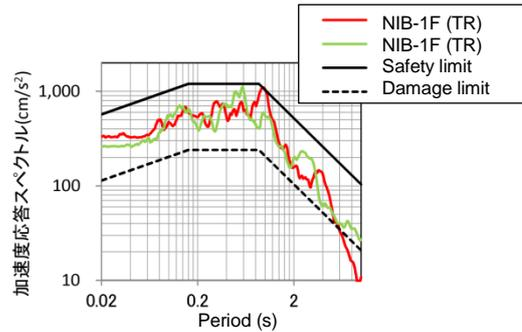
Figure 3.3. Acceleration response spectra at the first floor of the NIB
