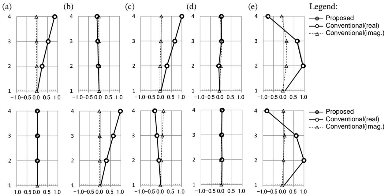
Figure 4.5. Comparison of singular vector and eigenvector at Location NW: (a) 2.26Hz, (b) 2.59Hz, (c) 3.44Hz, (d) 8.25Hz, and (e) 9.58Hz (upper figure for *TR* direction and lower figure for *LG* direction)
