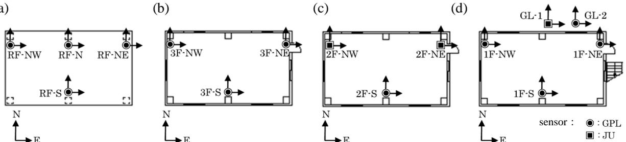
Figure 4.1. Location of portable accelerometers in the simultaneous array measurement :
