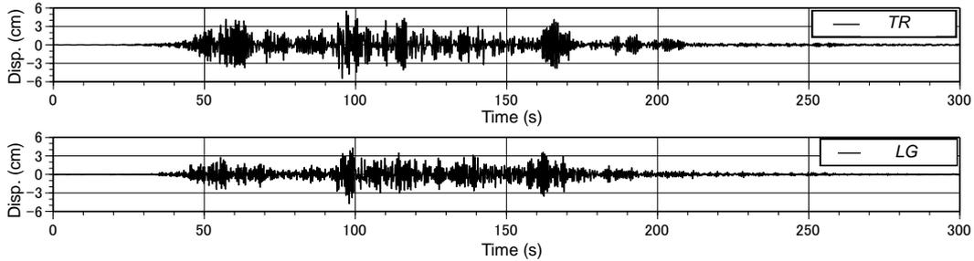
Figure 3.6 Calculated relative displacements at roof to the first floor (NIB)
