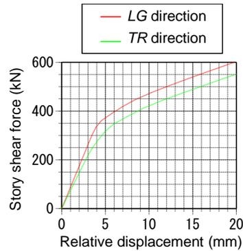
Figure 5.2. Relationship between story shear force and relative displacement (push-over analysis)
