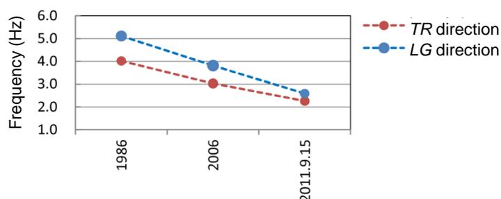
Figure 5.1. Change in the first natural frequency estimated from ambient vibration
