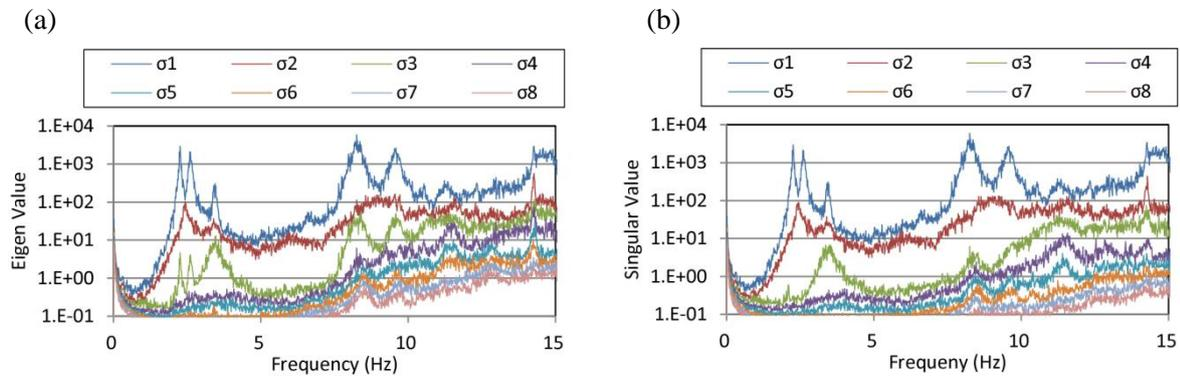
Figure 4.4. Comparison of singular value spectrum and eigenvalue spectrum: (a) singular value spectrum (conventional method), (b) eigenvalue spectrum (proposed method)
