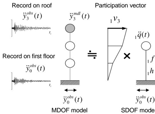
Figure 3.7. Schematic diagram of system identification using modal model
