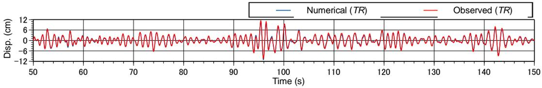
Figure 3.5. Validation of numerical integration using the observed records on IB (relative displacement of isolated layer)
