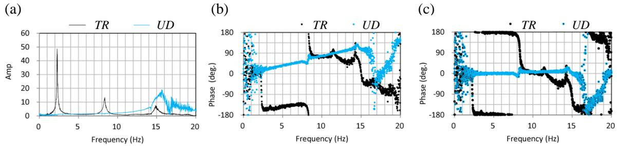
Figure 4.3. Frequency response function on the roof for the first floor (Location S): (a) amplitude of FRF, (b) phase of FRF before time correction, and (c) phase of FRF after time correction
