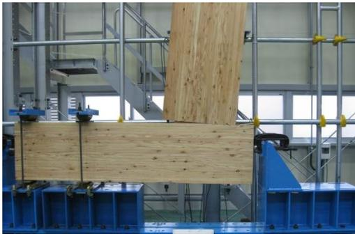
1) Beam's butt end embedding in the column
