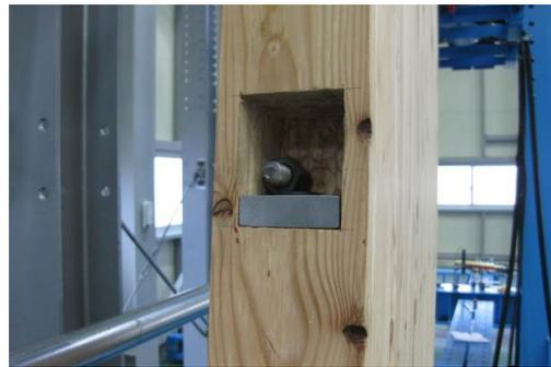
2) Tension side anchor-bolt elongation and rupture
