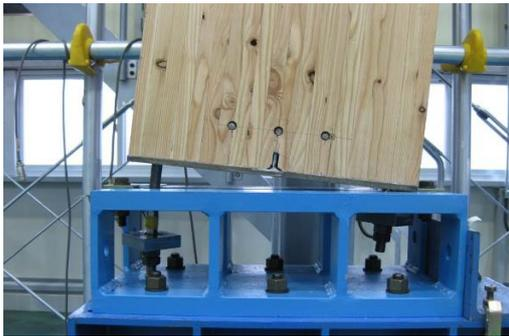
1) Tension side anchor-bolt elongation
