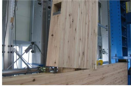
2) Beam's butt end embedding in the column
