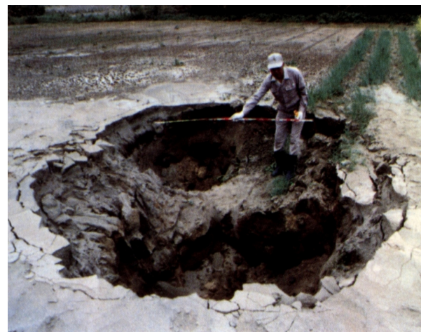
Photo 2 Large sand boil [Reference 9)]
