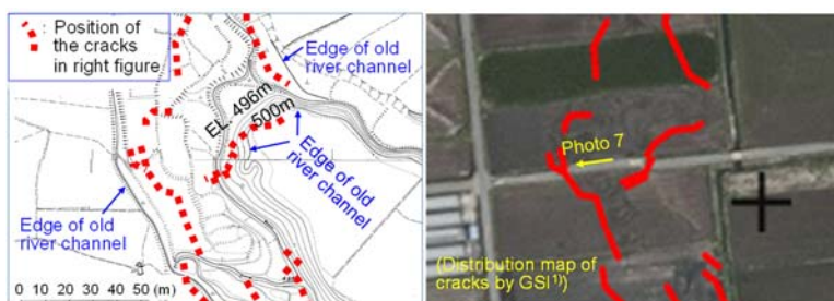
Fig. A1 Position of cracks on old topographic map of the Yakuimbaru district
