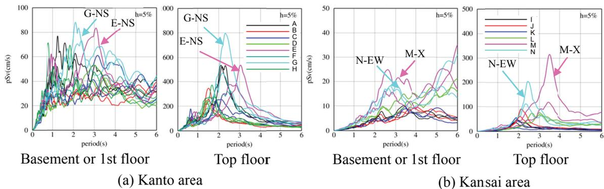
Fig.3 Pseudo velocity response spectra of recorded motions in super high-rise residential buildings
