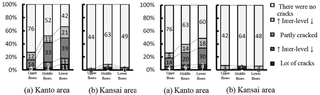
Fig.20 Cracks in interior materials
