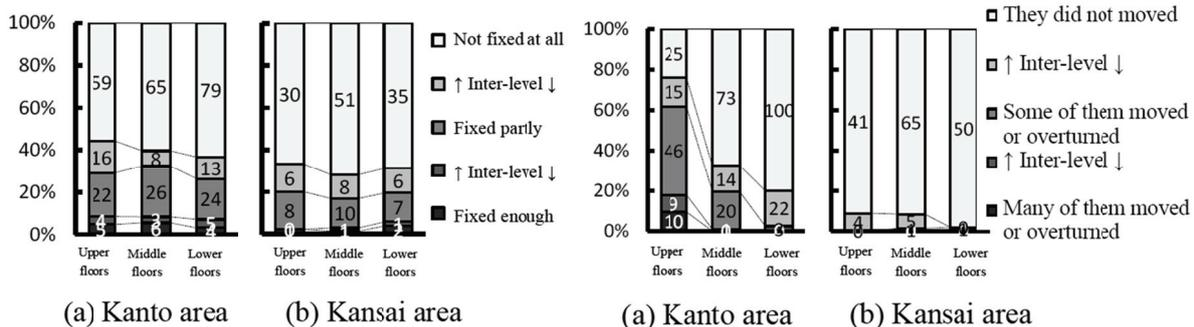
Fig. 16 Fixing condition of drawers, refrigerators or cupboards
