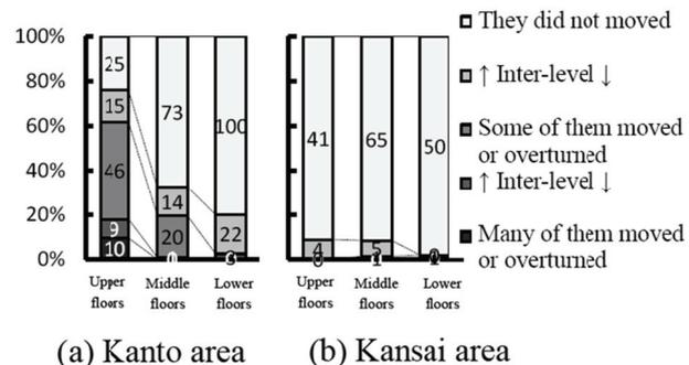
Fig. 17 Situations of drawers, refrigerators or cupboards after the main shock
