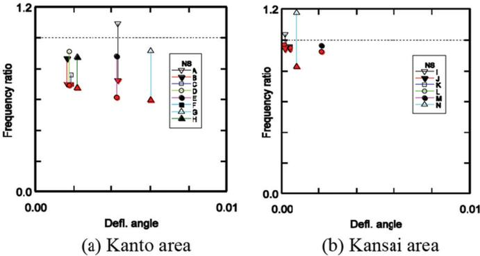
Fig.9 Minimum frequency ratios of all buildings during the 3.11 main shock (NS direction)
