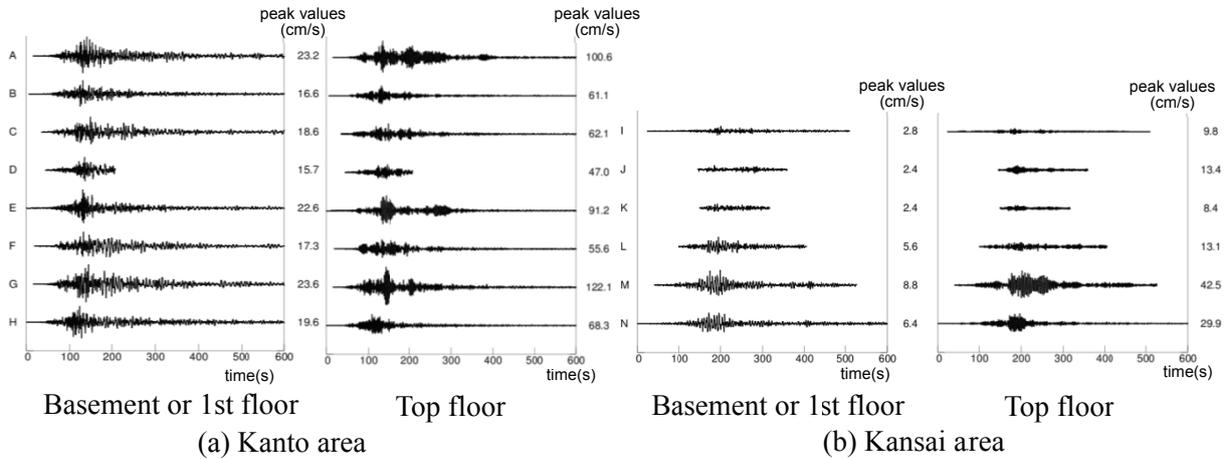
Fig.2 Velocity waveforms of recorded motions in super high-rise residential buildings
