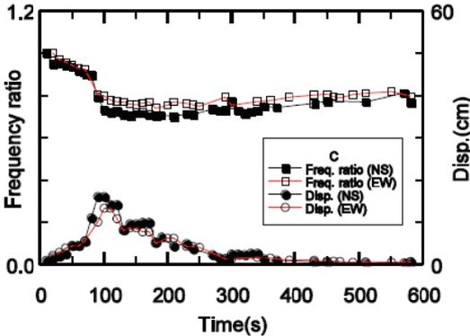
Fig.8 Temporal variation in the fundamental predominant frequencies in Building C during the 3.11 main shock
