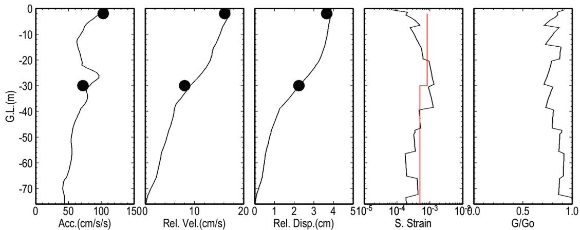
Fig.11 Depth distribution of maximum response calculated by earthquake response analysis. A filled circle and red line had indicated observation results.
