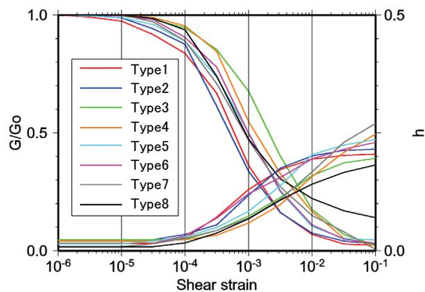
Fig.10 Nonlinear properties which are  $G/Go - \gamma$  and  $h - \gamma$  of each layers
