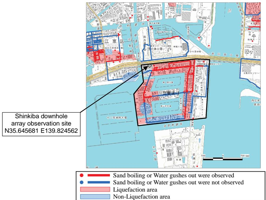
Fig. 4 Liquefaction investigation results around Shinkiba downhole array observation site after the 2011 off pacific of Tohoku earthquake (Revised Kanto regional bureau, MLIT and JGS 2011)
