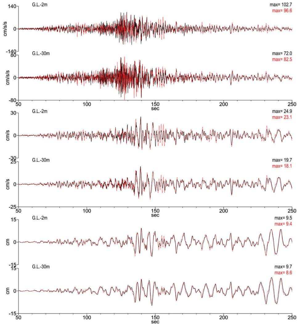
Fig. 12 Comparison of an observation waveform and an analysis waveform at G.L.-2m and G.L.-30m. A black line means observation and a red line means analysis.
