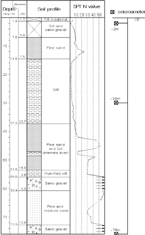
Fig. 2 Soil profile at Shinkiba site and installation depth of the seismometers.
