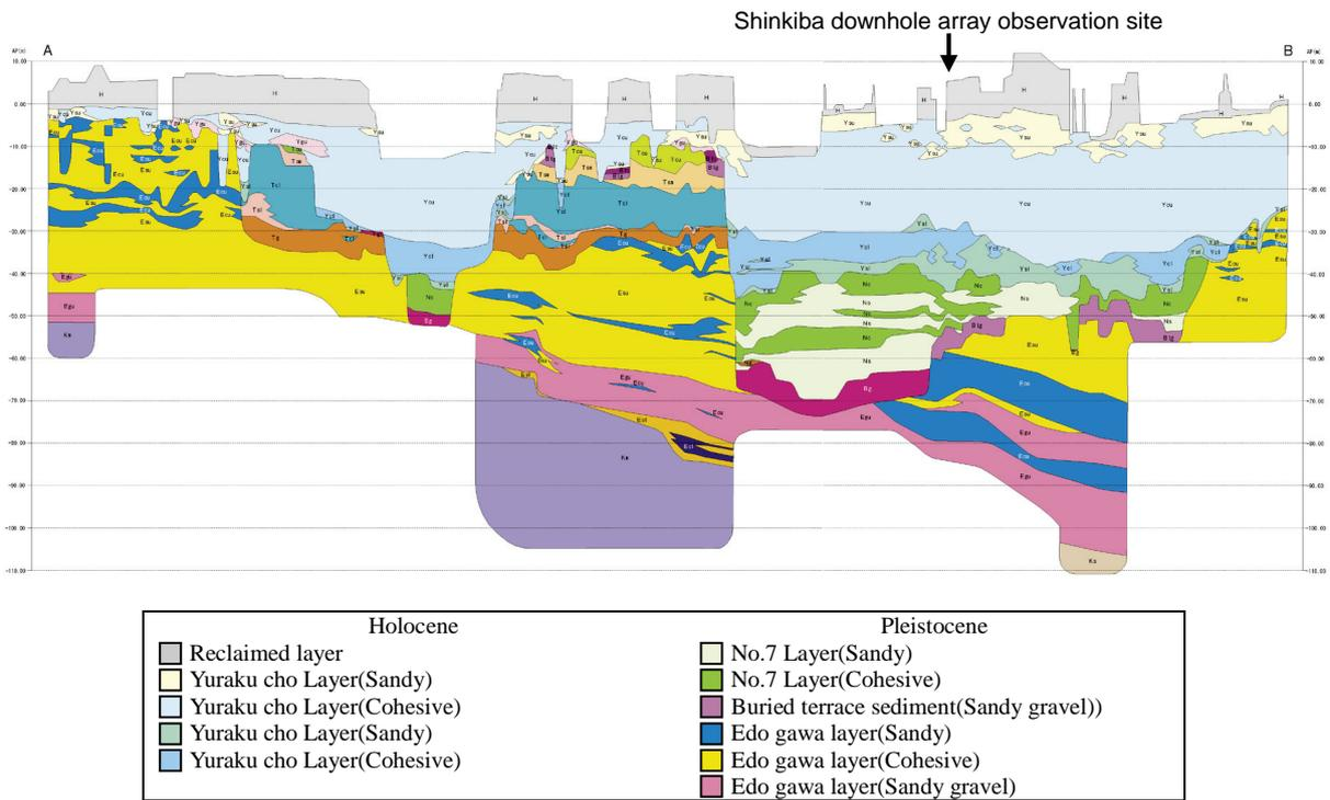
Fig. 3 Geological cross-section around downhole array observation site
