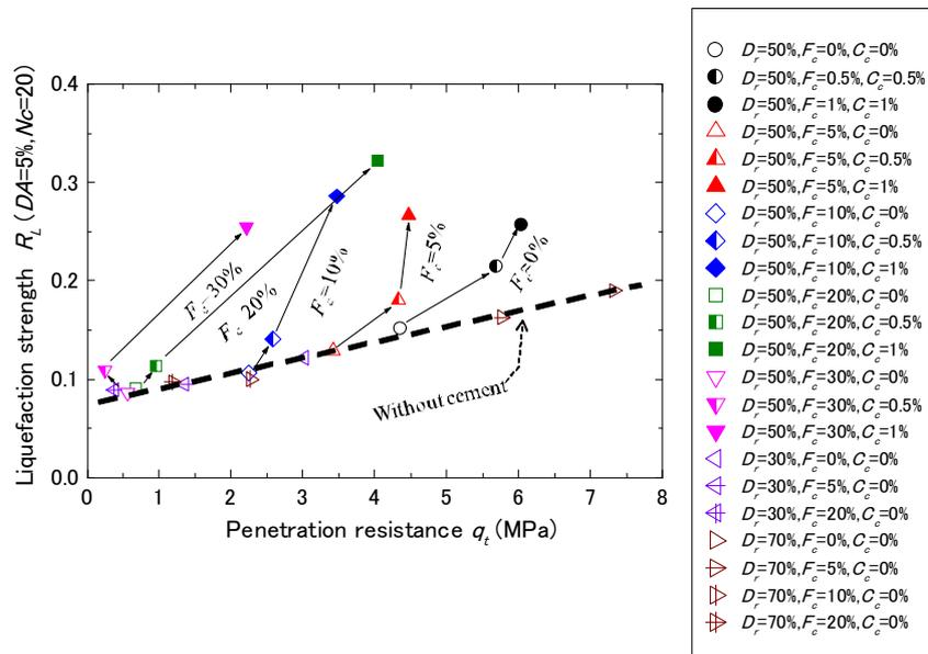
Fig. 6 Liquefaction strength  $R_L$  versus penetration resistance  $q_t$  diagram for different values of  $D_r$ ,  $F_c$  and  $C_c$ .
