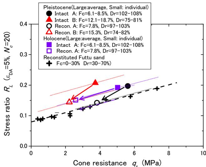
Fig. 13 Stress ratios  $R_L$  versus cone resistance  $q_t$  of intact Pleistocene and Holocene soils compared with reconstituted specimens.
