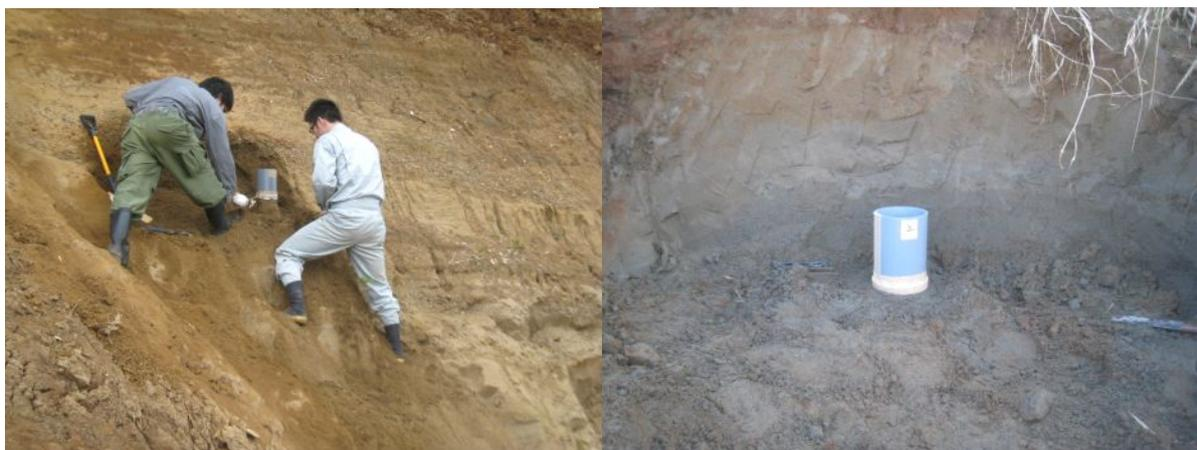
Fig. 10 Photographs of block sampling using a PVC tube with metal edge at the tip (Left: Pleistocene sand, Right: Holocene sand)
