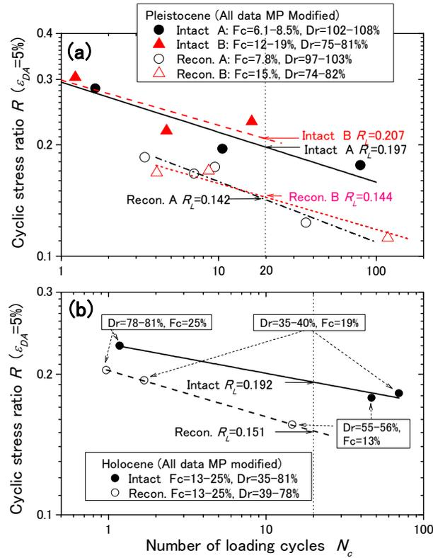
Fig. 12 Stress ratios  $R$  for  $\epsilon_{DA} = 5\%$  versus number of loading cycles  $N_c$  for intact specimens from Pleistocene sands.
