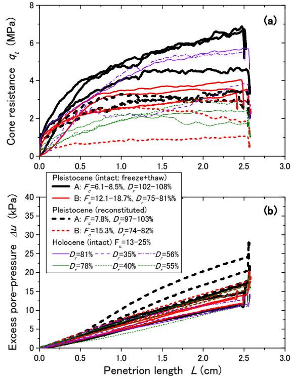
Fig. 11 Cone resistance (a) or excess pore- pressure (b) versus penetration length  $L$  for intact and reconstituted Pleistocene/Holocene sands.
