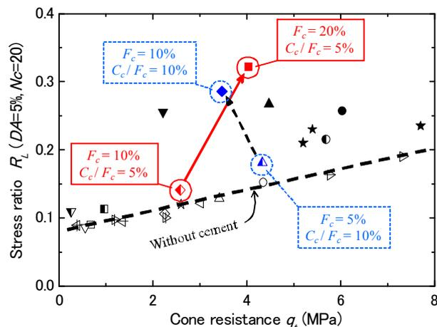
Fig. 9 Close-up of Fig. 6 showing the effect of fines content  $F_c$  for the same  $C_c/F_c$ .
