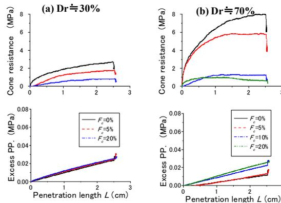
Fig. 3 Cone resistance or excess pore-pressure versus penetration length  $L$  for reconstituted specimens of  $D_r \approx 30\%$  &  $70\%$  with different fines content without cement.
