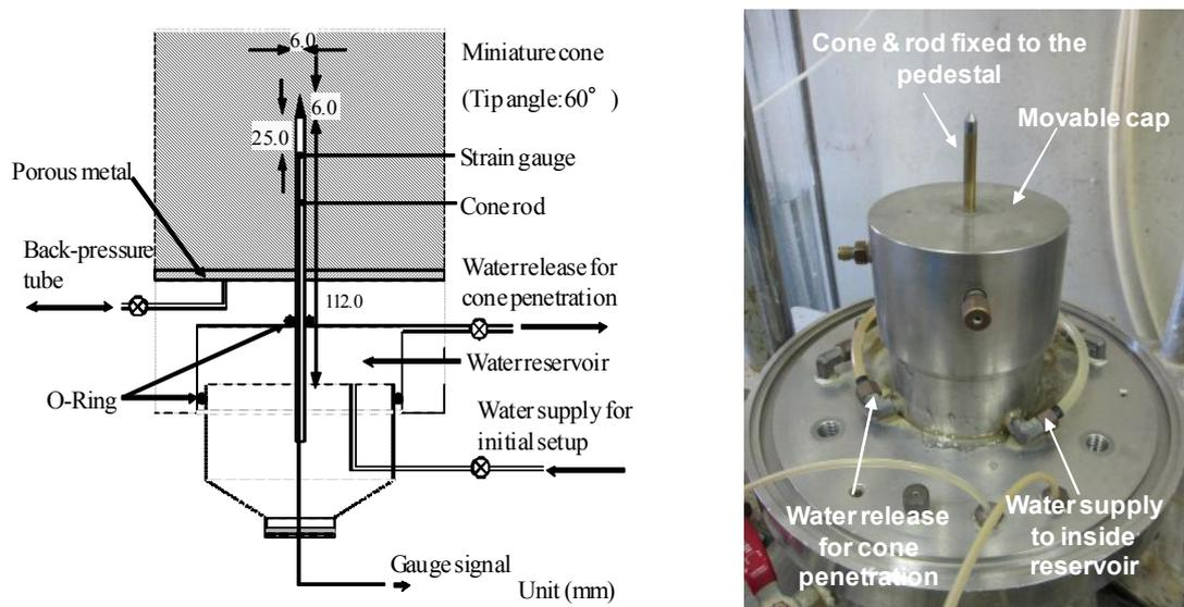
Fig. 1 Cross section (right) and Photograph (left) of the modified pedestal in the lower part of triaxial apparatus
