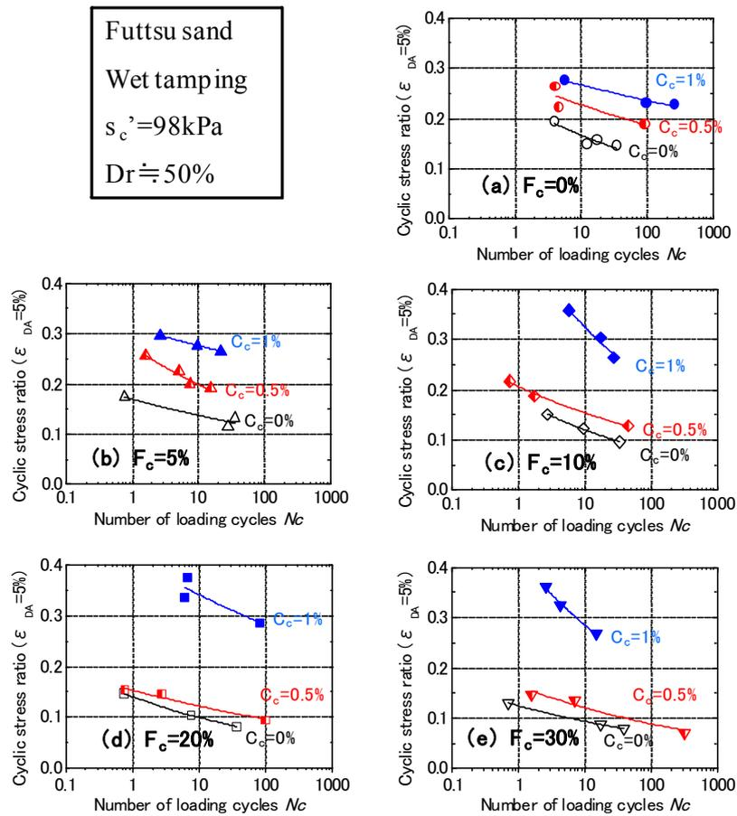
Fig. 4 Stress ratios  $R$  versus number of loading cycles  $N_c$  for reconstituted specimens of  $Dr \approx 50\%$  with different fines content.
