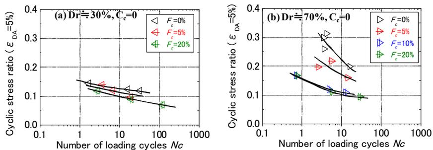
Fig. 5 Stress ratios  $R$  versus number of loading cycles  $N_c$  for reconstituted specimens of  $Dr \approx 30\%$  &  $70\%$  with different fines content without cement.
