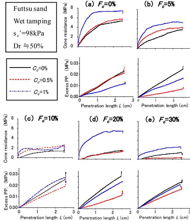
Fig. 2 Cone resistance or excess pore-pressure versus penetration length  $L$  for reconstituted specimens of  $D_r \approx 50\%$  with different fines content.
