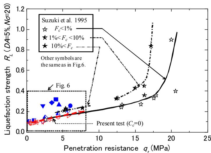
Fig. 7 Liquefaction strength  $R_L$  versus penetration resistance  $q_t$  compared with field investigations combining prototype CPT and triaxial tests on intact samples.
