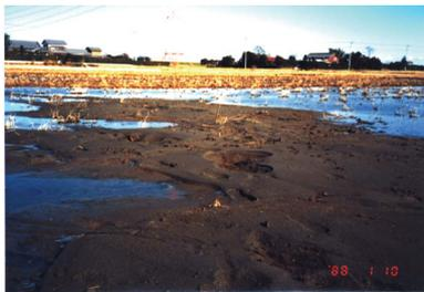
(a) 1987 sand boils from fissures near B-2 in Fig 6 (a)
