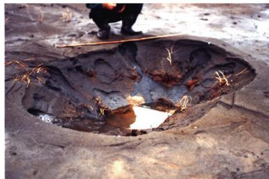
(b) 1987 sand boils crate near B-4 in Fig 6 (a)
