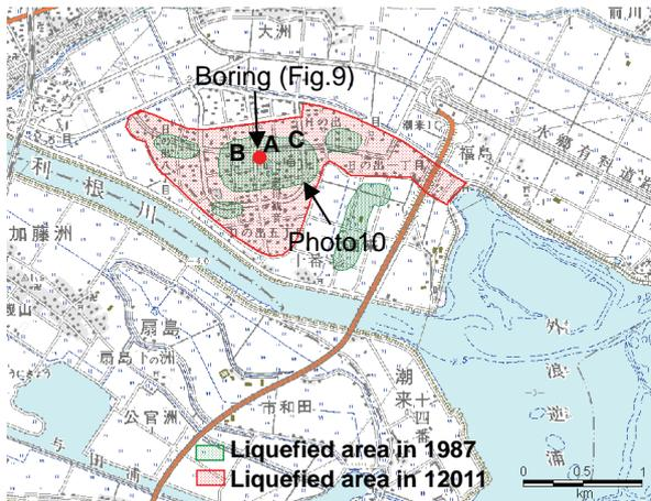
Fig. 8 Areas of liquefaction in Hinode of Itako City during the 1987 and 2011 earthquakes
