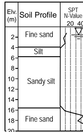
Fig. 9 Soil profile and SPT N-value in Hinode, Itako City (see Fig. 8 for location)
