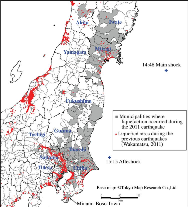
Fig. 1 Distribution of cities, special wards, towns, and villages where liquefaction occurred during the Great East Japan earthquake and liquefied sites in past earthquakes
