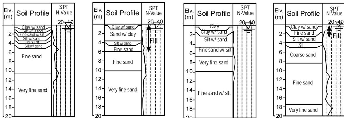
(a) B-1 (Minor sand boils in 1987) (b) B-2 (Large amount of sand boils from fissures in 1987) (c) B-3 (No effect of liquefaction in 1987) (d) B-2 (Large amount of sand boils from craters in 1987)
