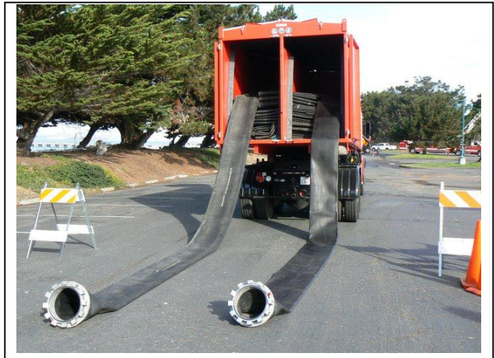
Figure 9 Berkeley FD 12” (30 cm) Aboveground Water Supply System (BAWSS)
