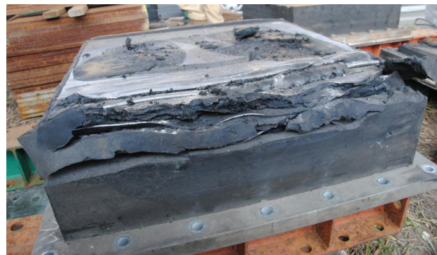
(b) Rupture of an elastomeric bearing
