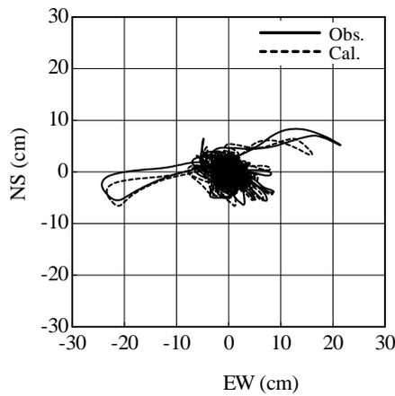
Fig. 17 Comparison of orbit of relative displacement
