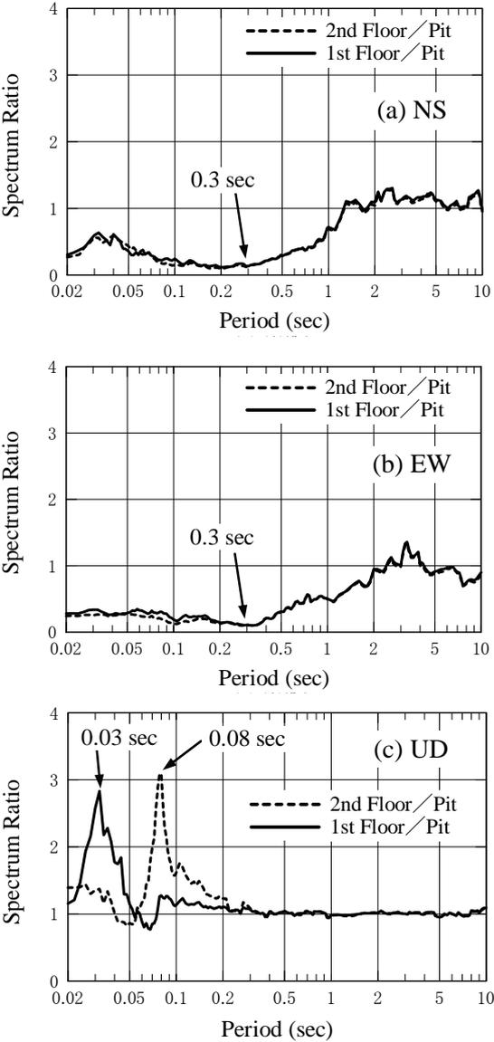
Fig. 7 Response spectrum ratio of the floor vs basement pit
