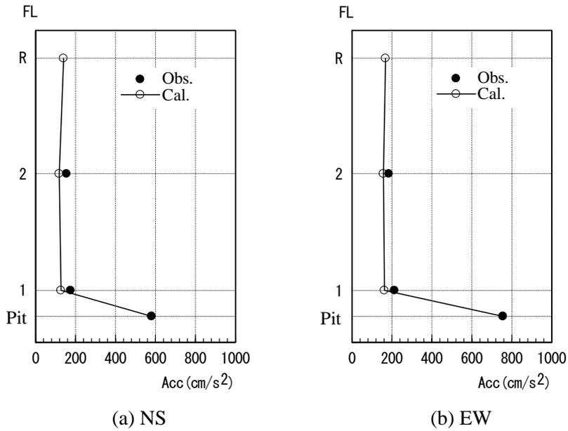
Fig. 12 Comparison of simulated peak acceleration and observed one
