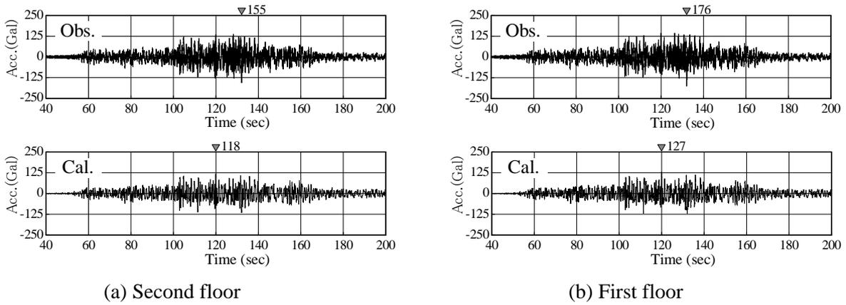
Fig. 13 Comparison of simulated time histories and observed one (NS)
