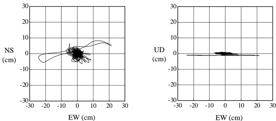
Fig. 9 Orbit of relative displacement between first floor and basement pit
