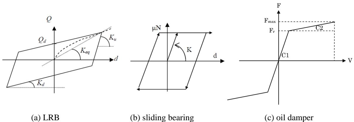
Fig. 11 Nonlinear hysteresis characteristics of devices
