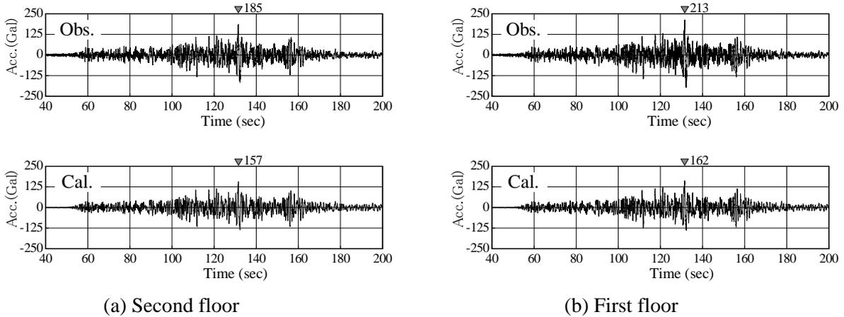
Fig. 14 Comparison of simulated time histories and observed one (EW)
