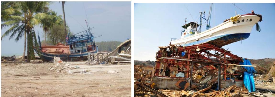
Fig. 4 Tsunami induced transport and deposition of vessels in Thailand 2004 (Intensity: VIII-IX) and Japan 2011 (Intensity: XI-XII).
