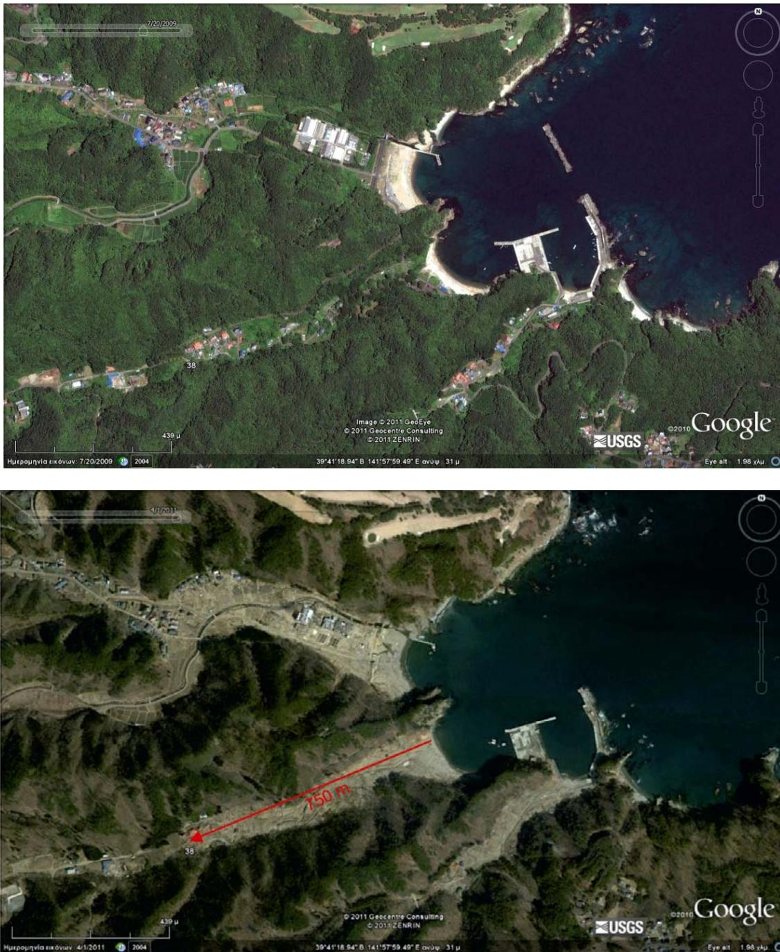
Fig. 5 Satellite imagery before and after the 2011 Tsunami, showing the effects on coastal areas, about 5km of Miyako town, in Onatsume area. Inundation was estimated at 750m and Runup at 37m. Damage in port facilities, infrastructure, houses and industrial facilities etc., are visible, as well as effects in natural environment (Intensity: XII).
