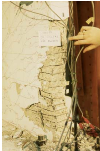
Fig. 3b Specimen TW2 web boundary failure (Thomsen and Wallace, 2004)
