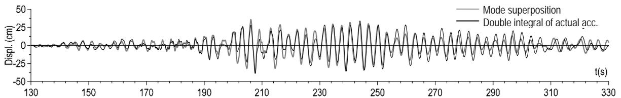
(c) Comparison: displ. obtained by mode superposition vs. double integral of recorded acceleration.
