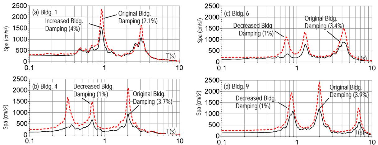
Figure 11. Component response spectra (component damping ratio = 3%).
