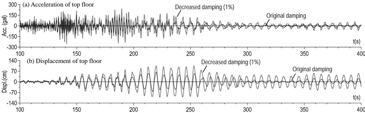
Fig. 10. Building 9 with different damping ratios (y-dir.).
