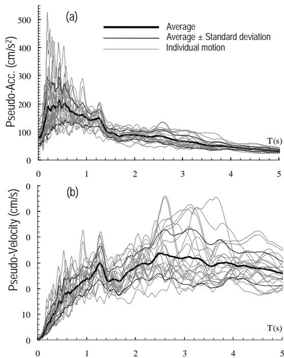
Fig. 1. Response spectra ((a) to (c)) generated from the base motions of the nine buildings (damping ratio 5%).
