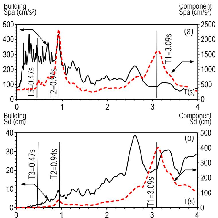
Fig. 4 Response spectra of Building 1 (solid lines) and component at top floor (broken lines).
