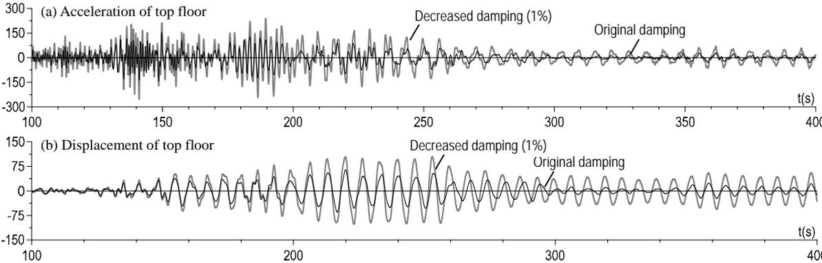
Fig. 8. Building 4 with different damping ratios (y-dir.).
