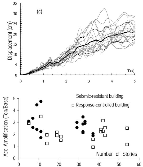
Fig. 2. Acceleration amplification factor vs. number of stories of buildings
