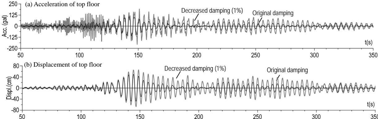
Fig. 9. Building 6 with different damping ratios (x-dir.).
