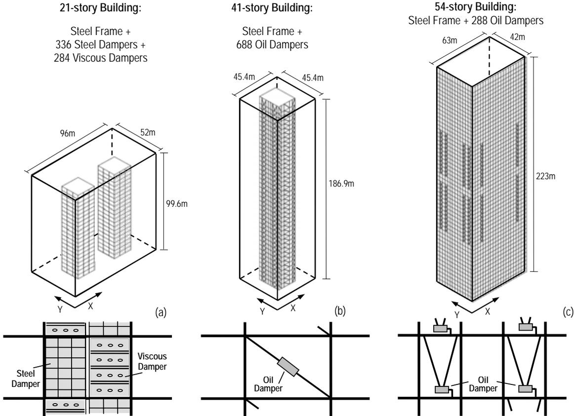
Fig. 7. Response-controlled buildings and dampers considered (Buildings 4, 6, 9 from left).
