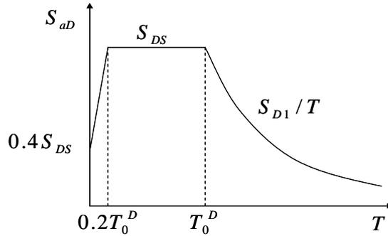
Fig. 11 Elastic acceleration response spectrum as the seismic demand for bridge to be retrofitted
