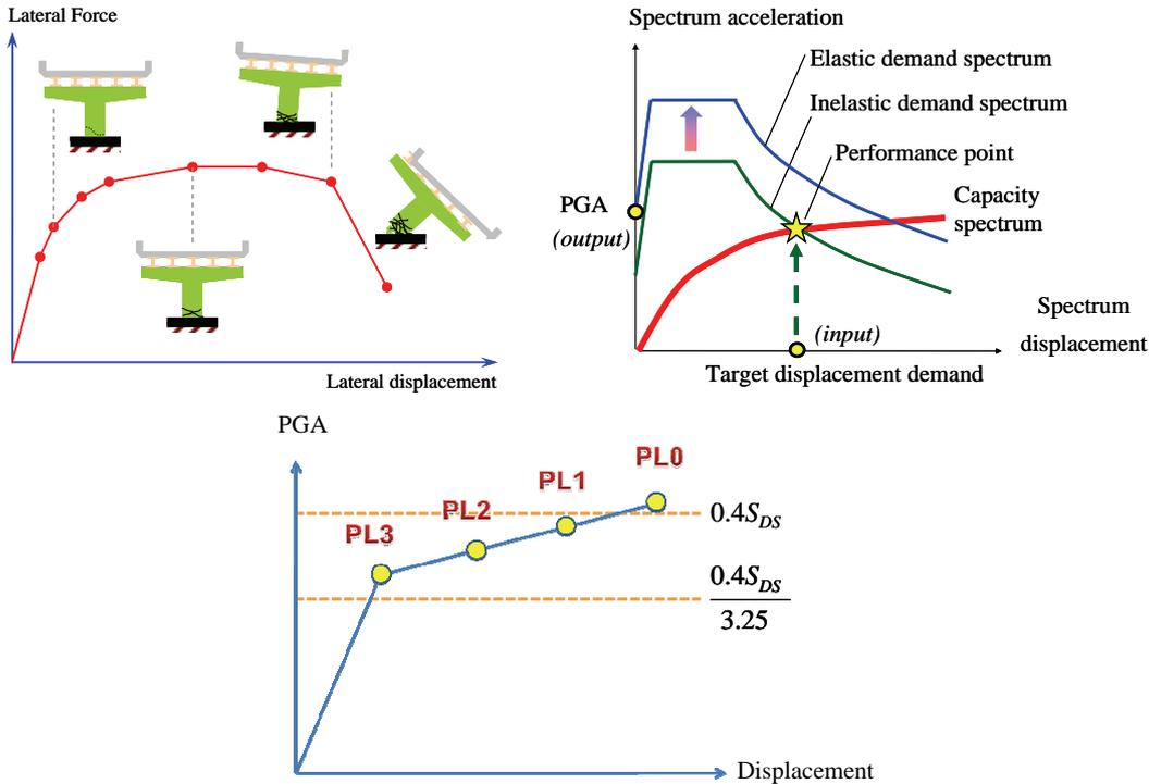
Fig. 13 Seismic assessment procedure and qualification requirement
