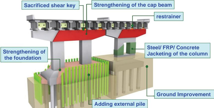
Fig. 15 Seismic retrofitting by using component approach
