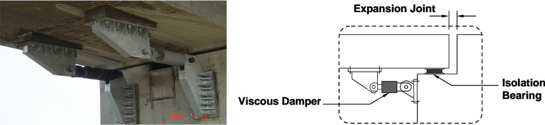
Fig. 14 Seismic retrofitting by using system approach: isolation bearing and external damper
