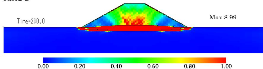
Fig.7 Distribution of accumulated plastic deviatoric strain
