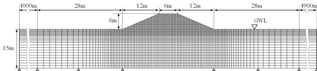
Fig.2 Finite element mesh and boundary conditions
