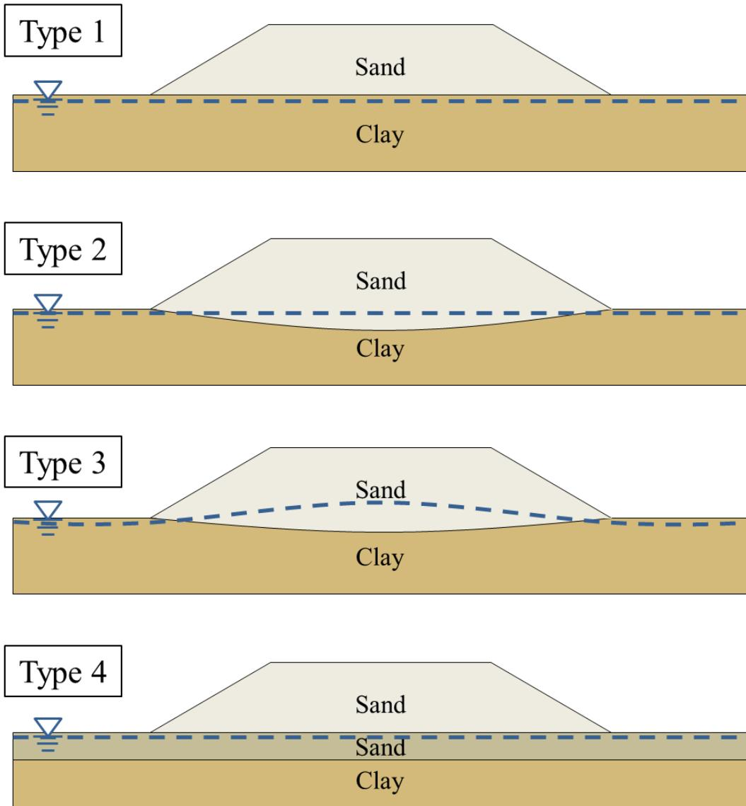
Fig.3 Soil profile and water table
