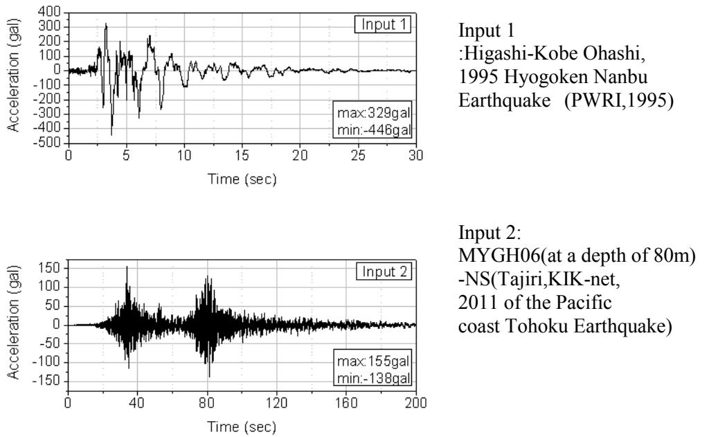
Fig.4 Input earthquake motions
