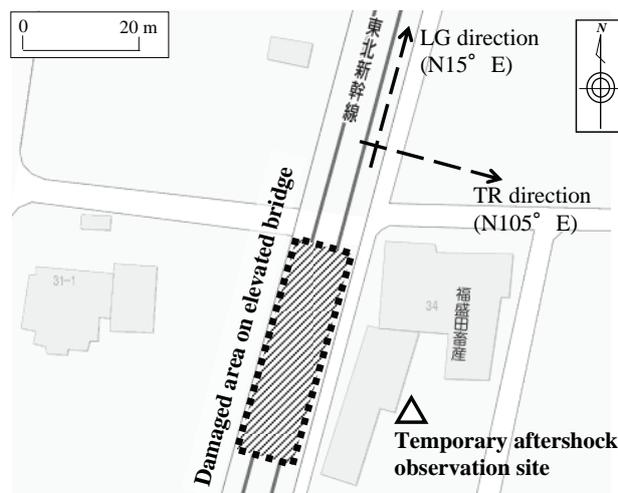
Fig. 6 Temporary aftershock observation site SNK
