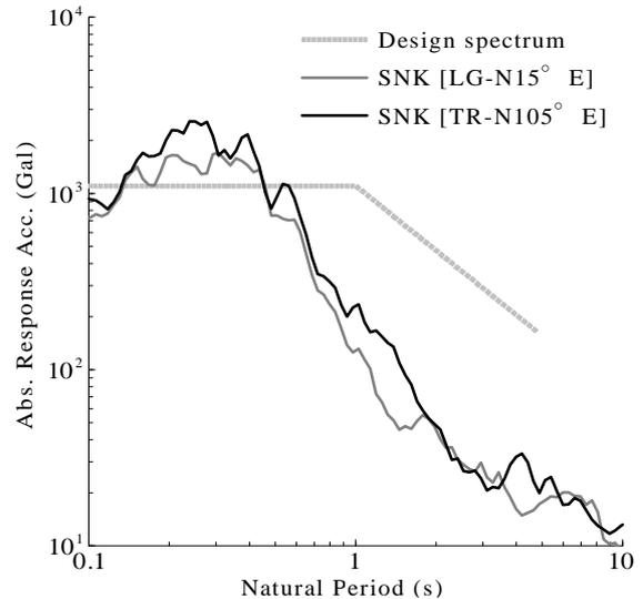
Fig. 13 The absolute acceleration response spectra
