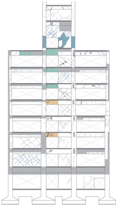
Fig. 4 Frame 10 cracks schedule
