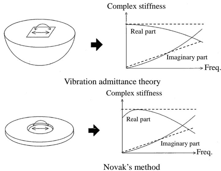
Fig. 4 Evaluation method of soil springs
