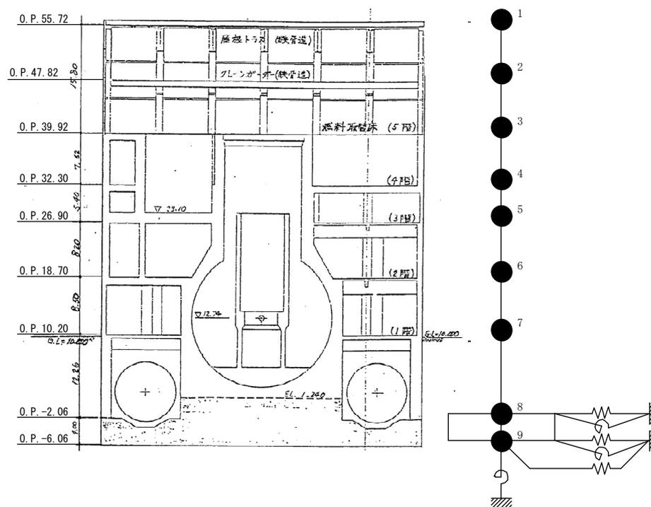
Fig. 3 Seismic response analysis model
