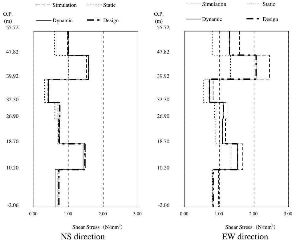
Fig. 8 Comparison of original design shear stress and that of simulation analysis
