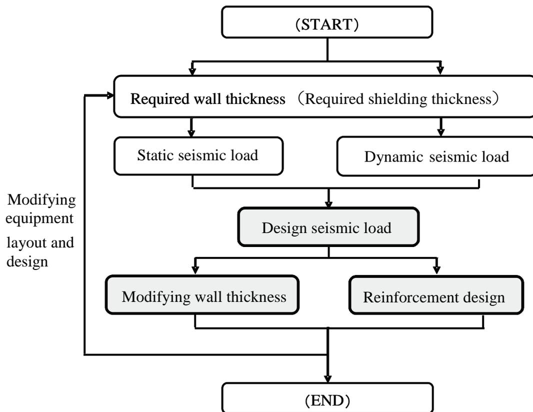
Fig. 7 Seismic design flow
