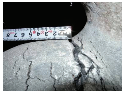
Fig. 21 Lead damper cracked
