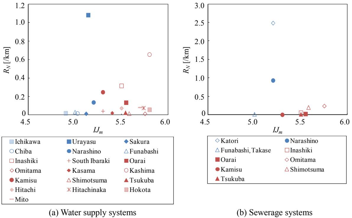
Fig. 2 Relation between damage ratio  $R_N$  and  $IJ_m$
