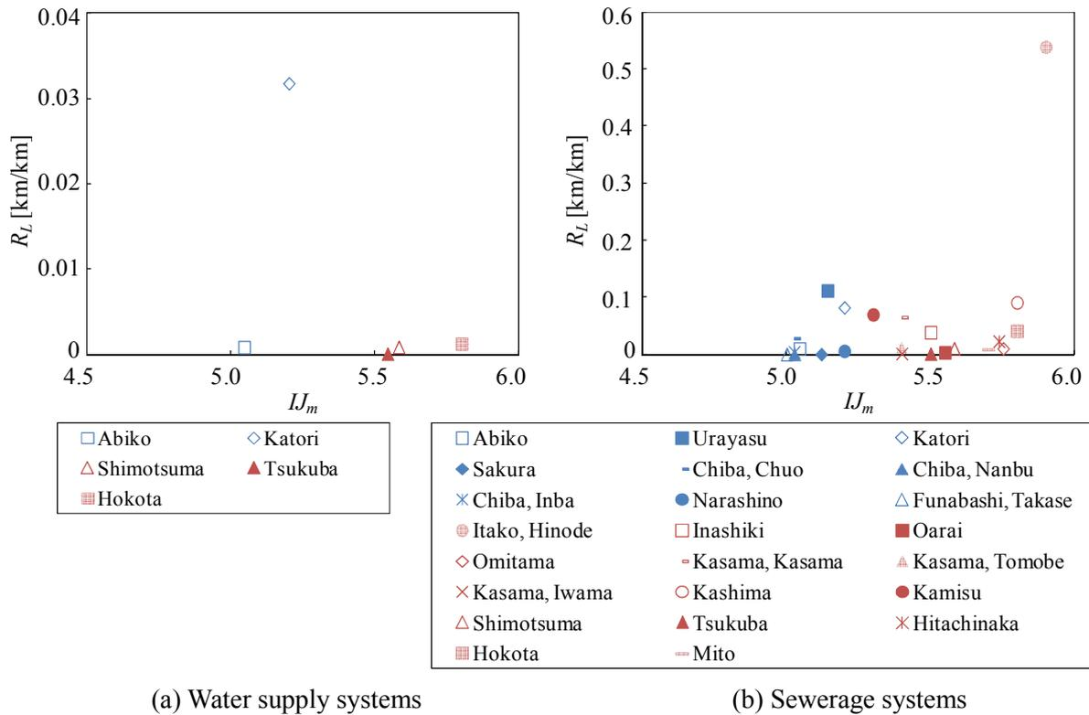
Fig. 3 Relation between damage ratio  $R_L$  and  $IJ_m$
