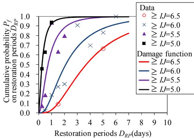
Fig. 10 Damage function on restoration periods  $D_{RP}$  with seismic intensity  $IJ$
