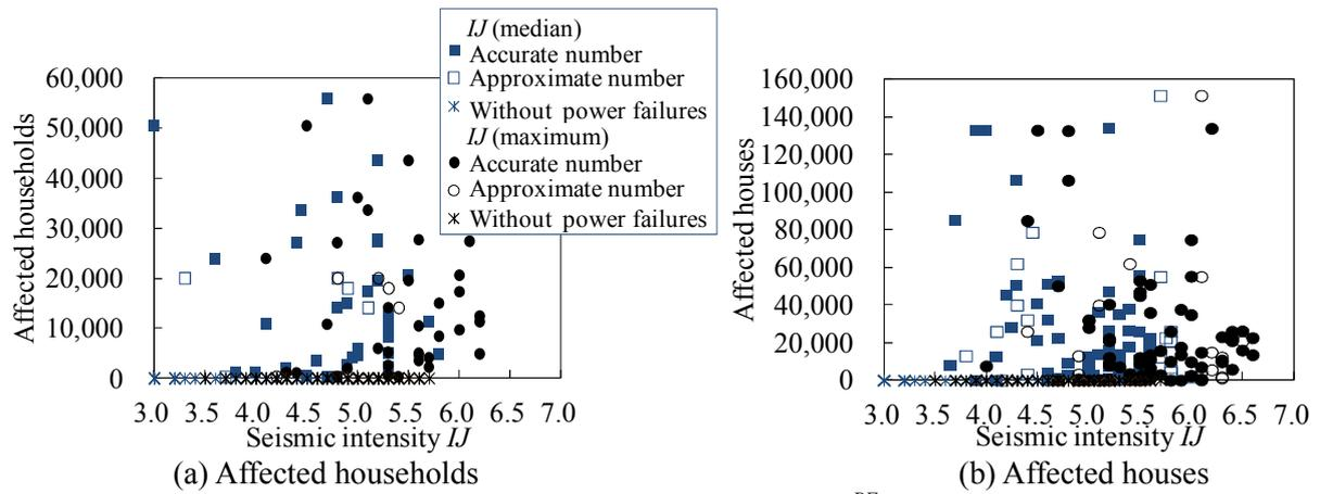
Fig. 4 Relation of the number of affected households and houses  $N^{PF}_i$  at a city  $i$  with seismic intensity  $IJ$
