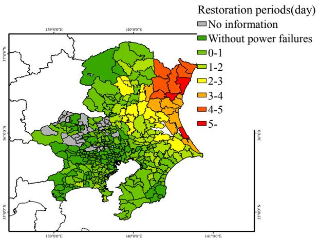
Fig. 9 Spatial distribution on restoration periods  $D_{RP}$  with seismic intensity  $IJ$
