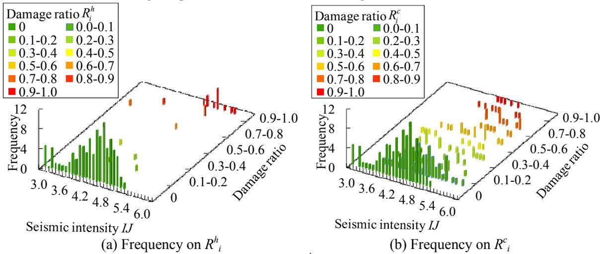
Fig. 7 Frequency of damage ratios  $R_i^h$  and  $R_i^c$  with seismic intensity  $IJ$
