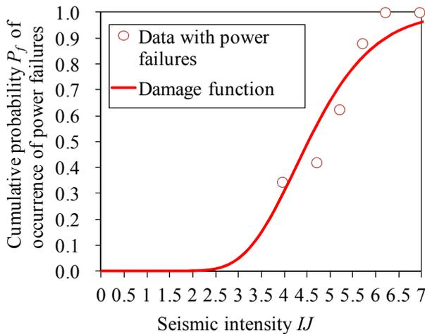
Fig. 3 Damage function on occurrence of power failures
