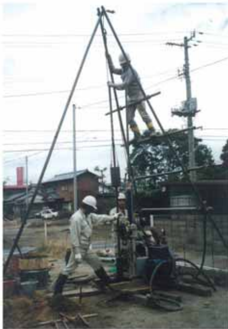
Fig. 4.1 Practice of Standard Penetration Test in Japan and USA
