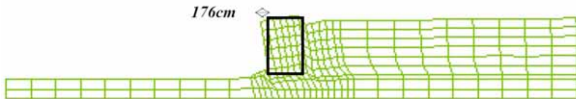
Fig. 2.55 Computed post-earthquake deformed shape for the quay wall without cartonplast
