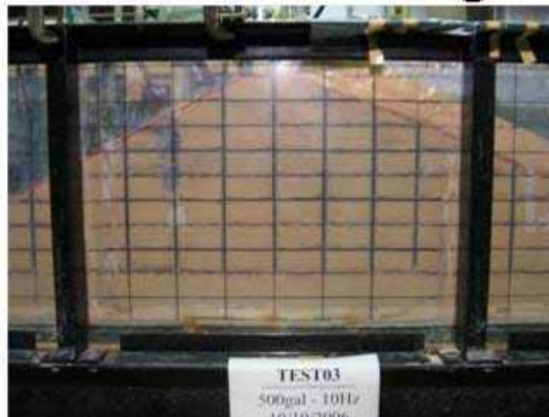
Fig. 2.22 Shape of surface lining dam after shaking
