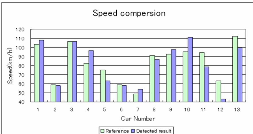
The standard deviation of the speed difference between the reference value and detected results is around **11km/h**.
