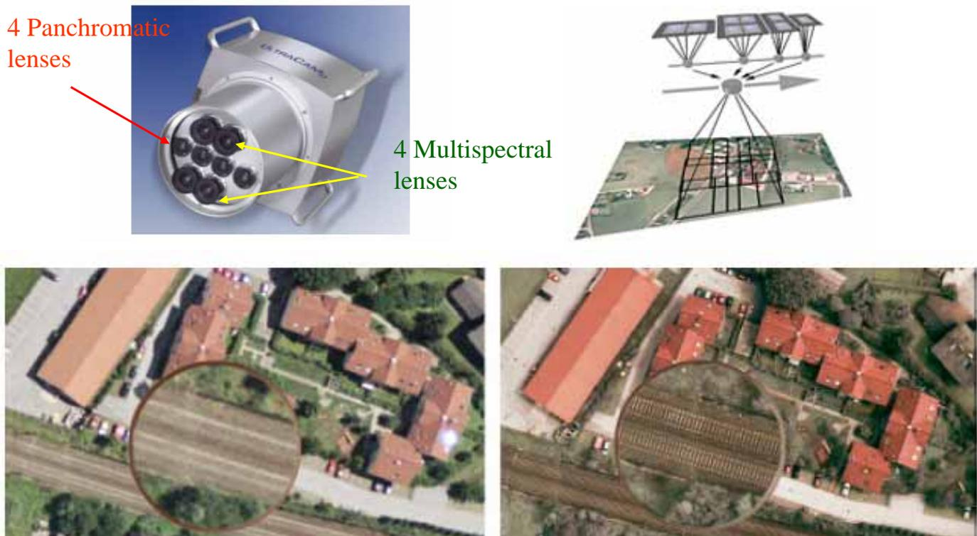
**Figure 6:** Color image segment from aerial film (left) with a GSD of 15 cm, obtained from a 12.5 $\mu$ m scan. The UltraCam-image has a GSD of 16 cm (right). The inserts are 2x enlarged and have a diameter of 150 pixels. Note the definition of the railroad track.
