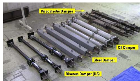
Fig. 2 Full-scale Dampers Tested Prior to Building Experiments
