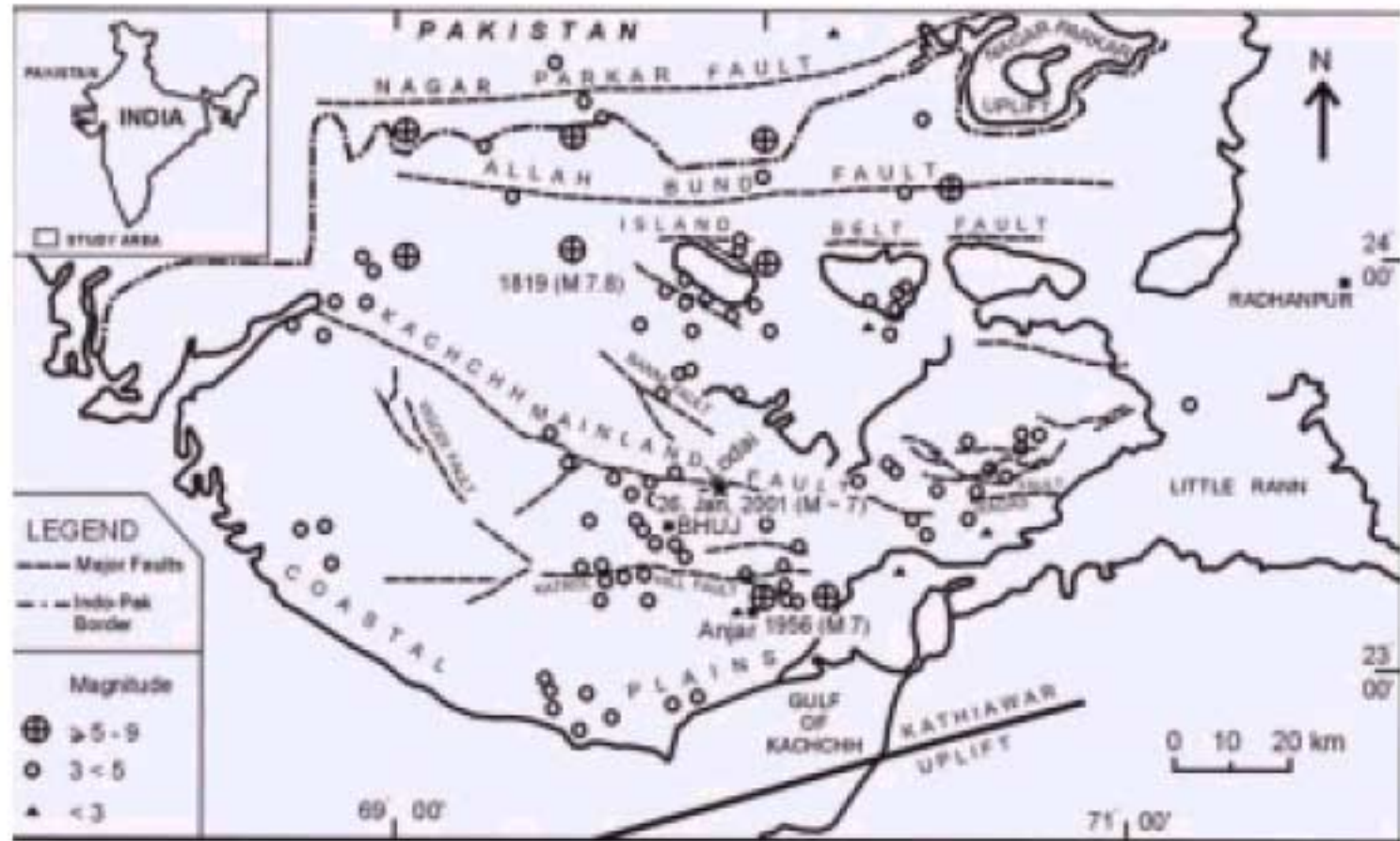
Figure 6 Spatio-Temporal distribution of earthquakes in Kutch region (Malik et al, 2000)
