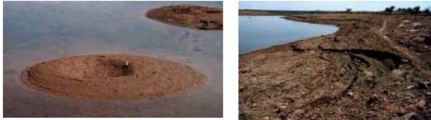
Figure 25 Liquefaction and lateral spreading at Chang dam
