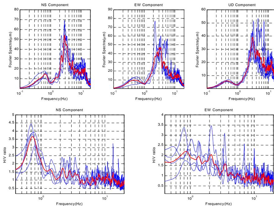
**Fig. 21.** Fourier spectra of microtremors at the toe of El Balsamo ridge
