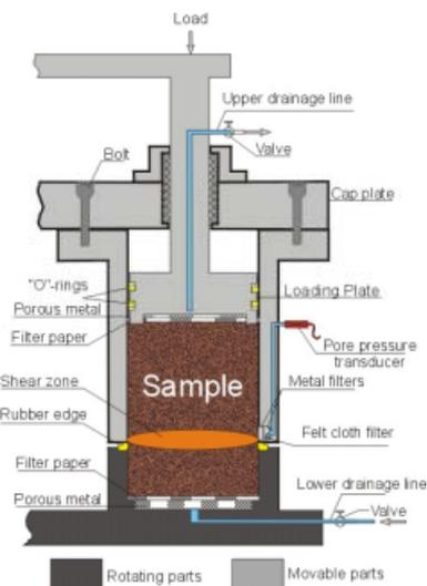
**Fig.18.** Cross-section (right half) of undrained ring shear box (Sassa, 2000)
