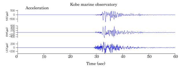
Figure 3. The 1997 Hyogo-ken-Nanbu earthquake's strong motions obtained by JMA 87-type electromagnetic strong motion seismograph.
