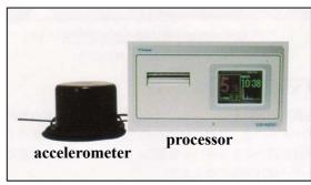
Figure 1. The picture of JMA 95-type seismic intensity meter. The left-hand side is an accelerometer and the right-hand side is an processor.
