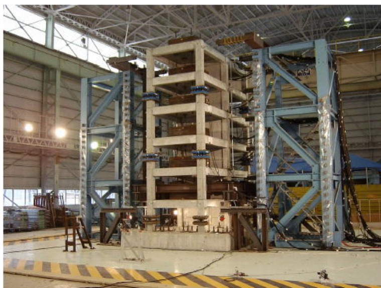
Photo 2 Preliminary shake table test for RC wall-frame structure – March 2003
