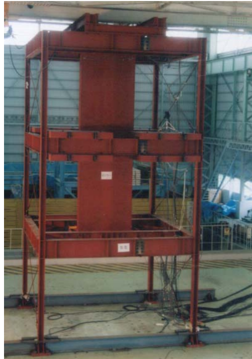
Photo 4 Vibration Test of Boiler Structure
