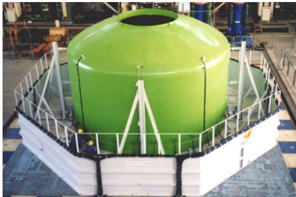
Photo 1 Vibration Test of Large Tank Model
