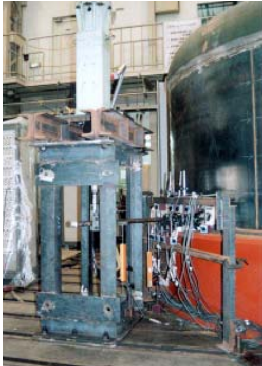
Photo 3 Collapse Test of Tank Nozzle
