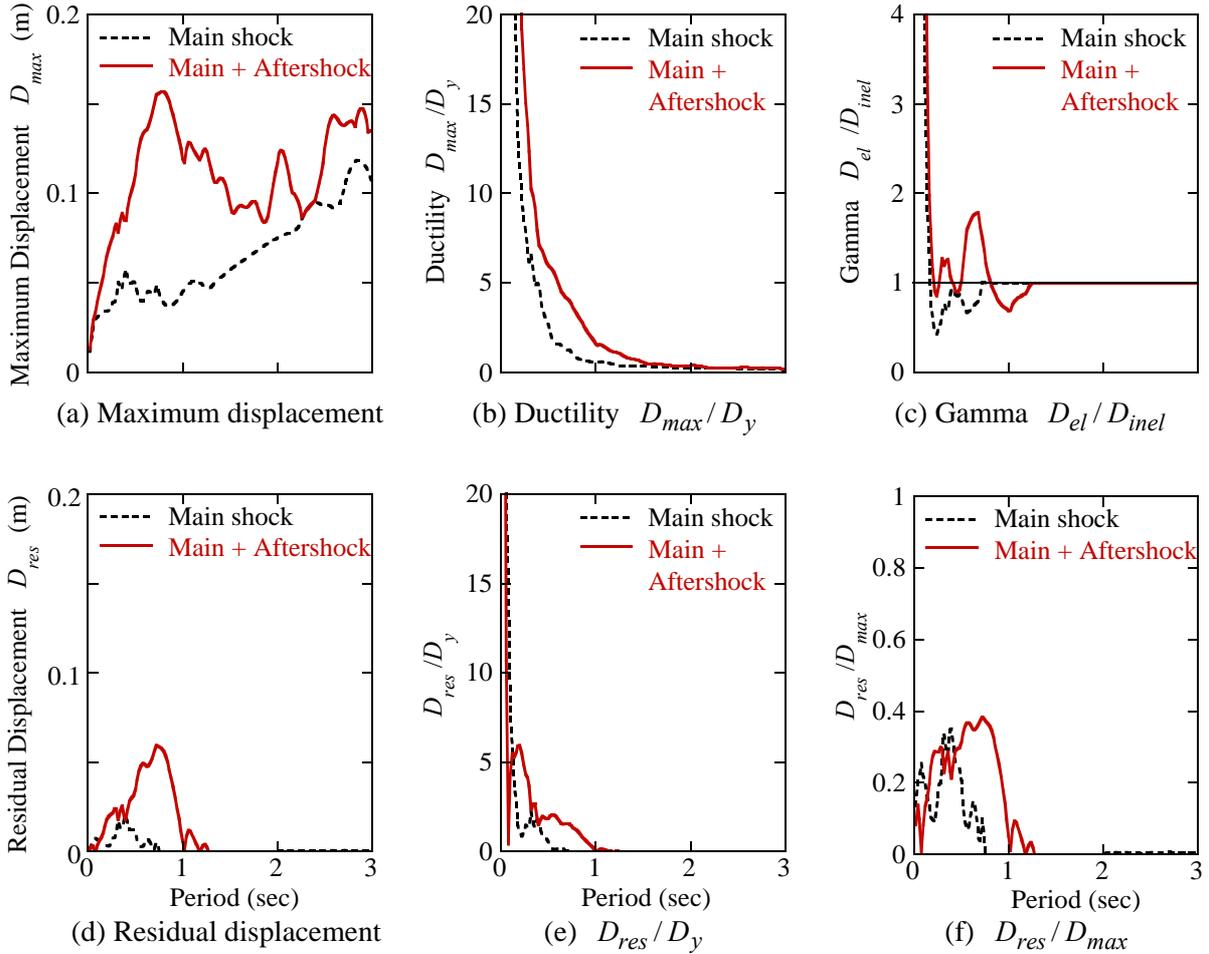
**Fig. 11** Effect of aftershock on nonlinear response spectra with  $a_y = 0.3$  g for NS component of Tohkamachi (NIG021) records
