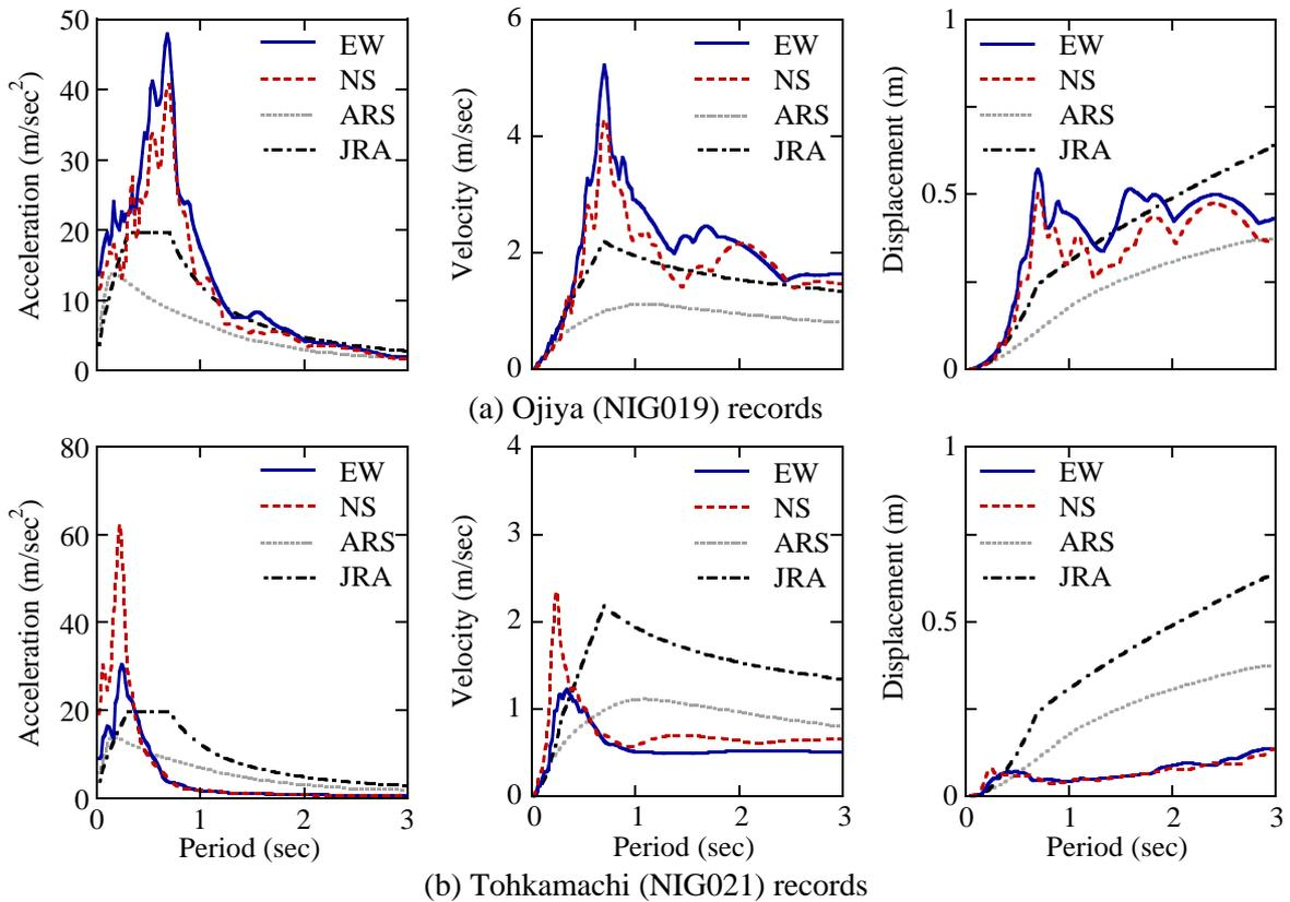
**Fig. 4** Elastic response spectra compared with design spectra
