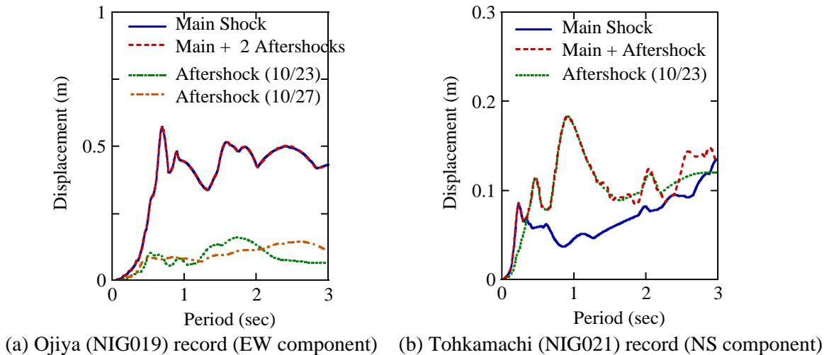
**Fig. 9** Effect of aftershocks on elastic response spectra
