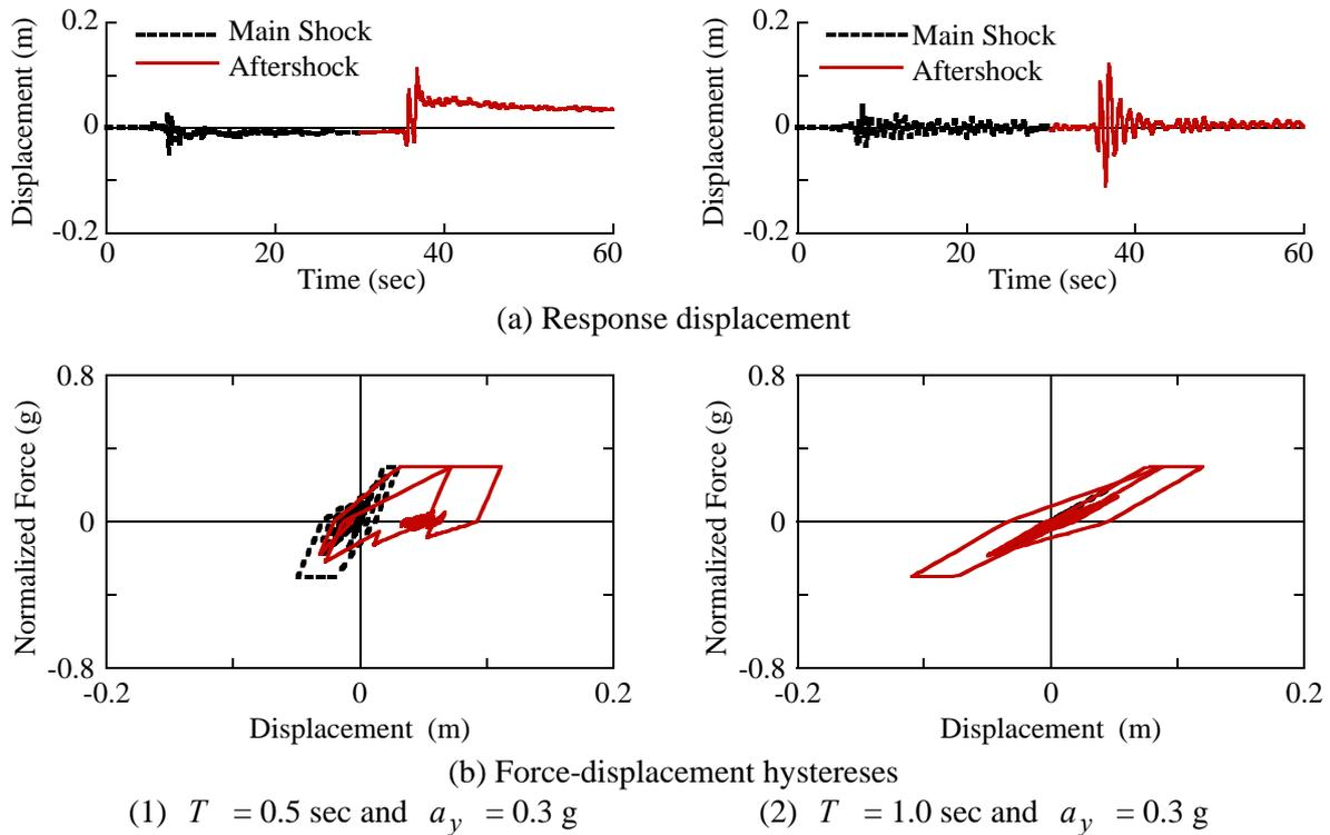
**Fig.10** Nonlinear dynamic response for combination of main shock and aftershock of NS component of Tohkamachi (NIG021) records
