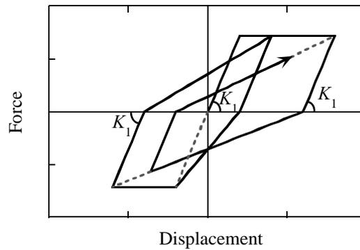
**Fig. 5** Stiffness degrading models
