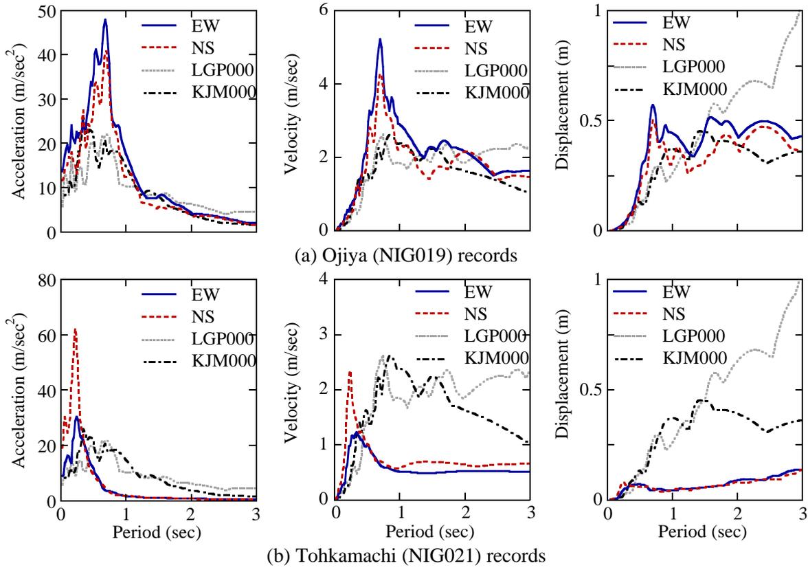
**Fig. 3** Elastic response spectra compared with past earthquake records
